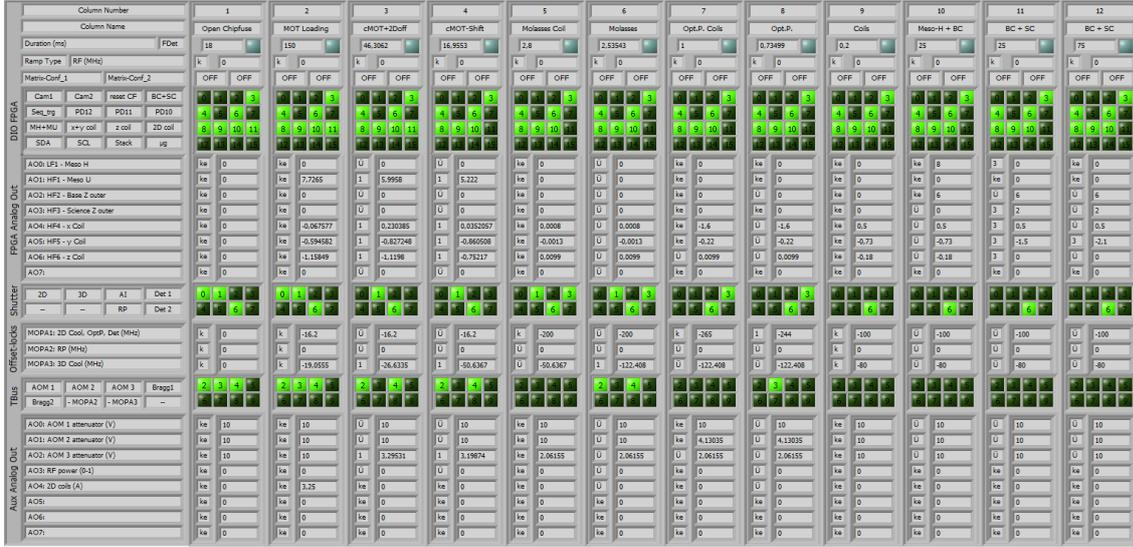
**Figure 2.15:** Control interface with the first part of an experimental sequence, which is uploaded to and executed by an FPGA. The columns constitute the smallest logical chunks within a sequence.
