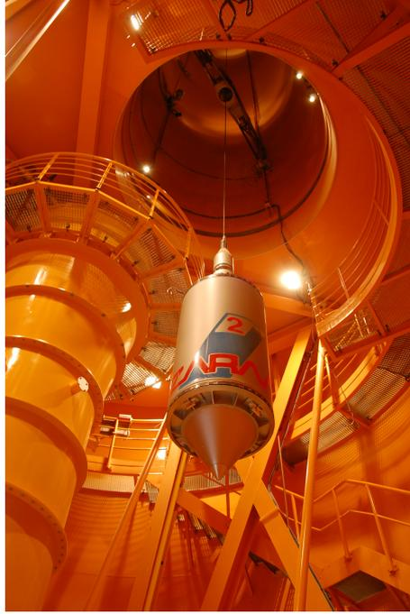
**Figure 1.3:** Drop capsule with the Q-2 experiment hanging inside the drop tower in Bremen next to the deceleration container, which is situated on the left side of the picture.
