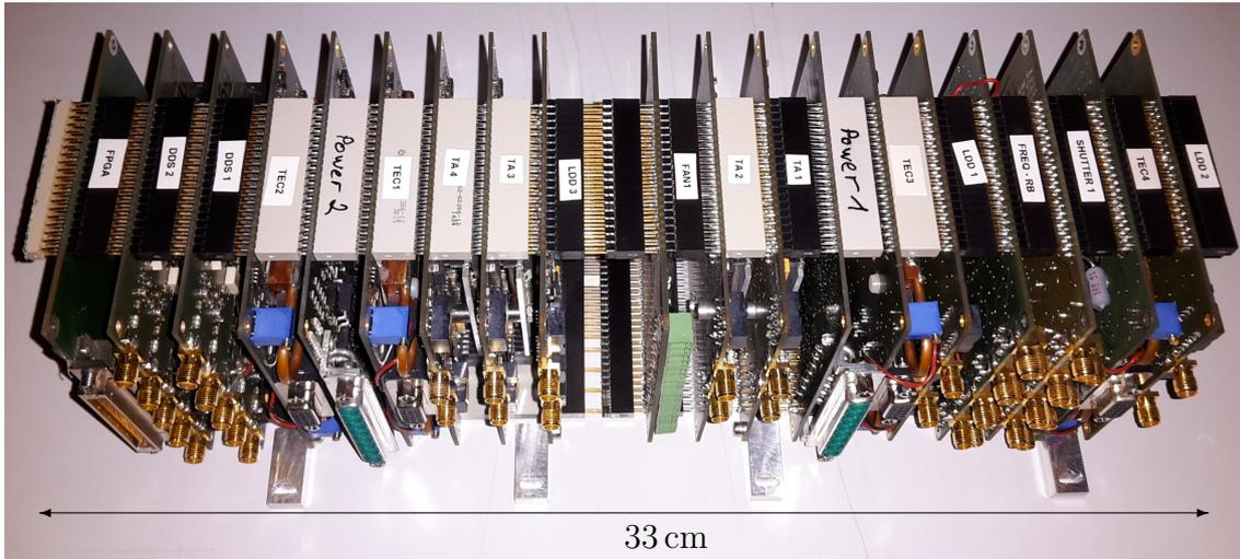
**Figure 2.14:** Customized electronics stack with laser current drivers, temperature controllers, locking electronics, DDS cards for driving AOMs, shutter controllers, communication and power interfaces. All cards have been developed by Thijs Wendrich in Hanover.
