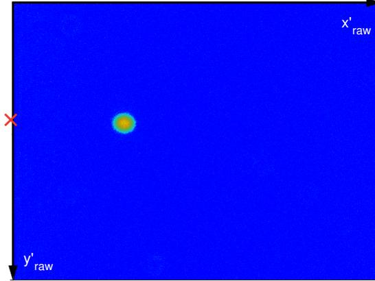
**Figure 2.9:** Atomic density image resulting from processing the atom and beam image in Fig. 2.8 using Eq. (2.9). The atomic ensemble (yellow region) was detected in microgravity 100 ms after releasing a Bose-Einstein condensate from its trap. The  $x'_{\text{raw}}$  and  $y'_{\text{raw}}$  axes show the camera coordinate system of the first detection system (Detection 1) and the red 'x' marks the origin of the Q-2 coordinate system.
