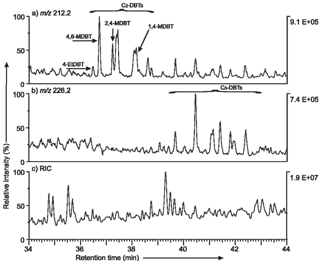
**Figure 5-25** Partial mass chromatograms of a) C<sub>2</sub>-dibenzothiophenes, b) C<sub>3</sub>-dibenzothiophenes and c) reconstructed ion current of the degraded Vienna basin oil; M: methyl-, Et: ethyl-, DBT: dibenzothiophene.
