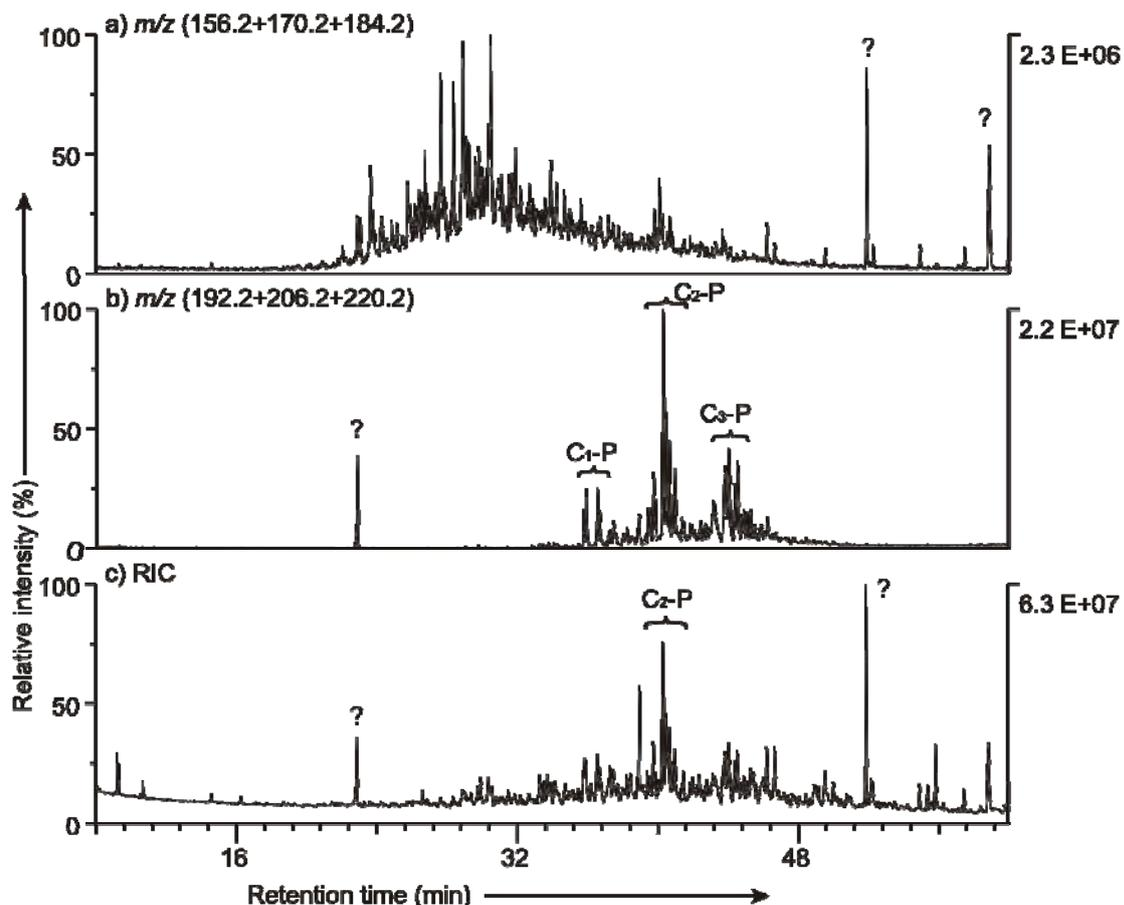
**Figure 6-5** Partial chromatograms of (a) molecular ions of C<sub>2</sub>- to C<sub>4</sub>-naphthalenes, (b) molecular ions of C<sub>1</sub>- to C<sub>3</sub>-phenanthrenes and (c) total ion current of accumulated compounds in sample Whv-II-dV-200b; P = phenanthrene, ? = unknown compounds.
