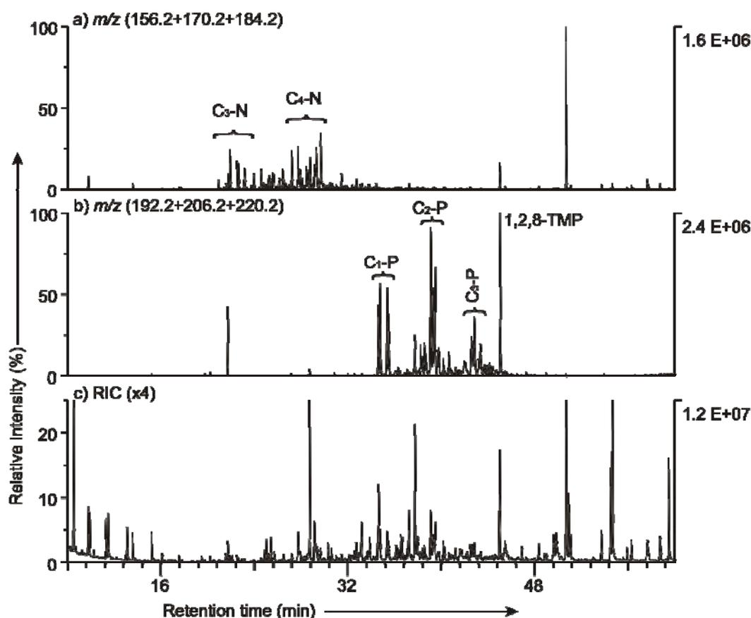
**Figure 6-1** Partial chromatograms of (a) molecular ions of  $C_2$ - to  $C_4$ -naphthalenes, (b) molecular ions of  $C_1$ - to  $C_3$ -phenanthrenes and (c) total ion current of accumulated compounds in mussels sample Ply-uM-200; N = naphthalene, P = phenanthrene, TMP = trimethylphenanthrene.
