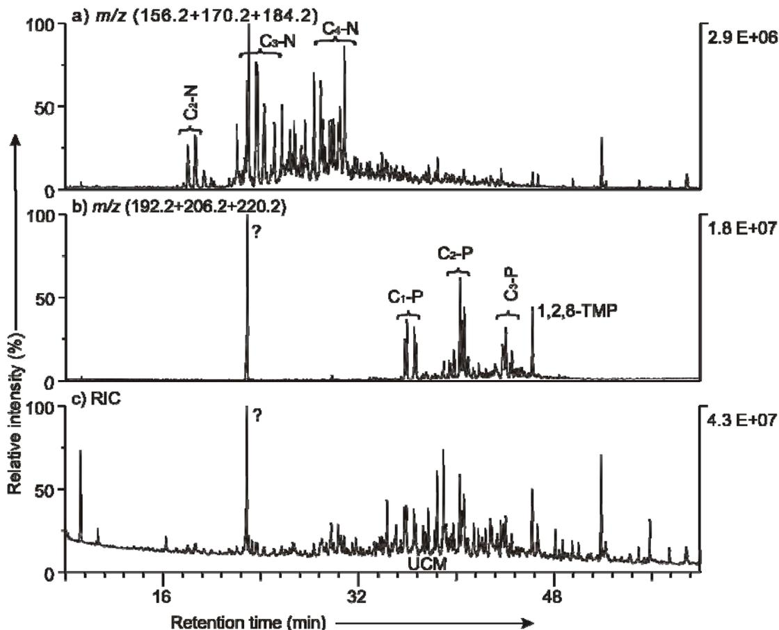
**Figure 6-3** Partial chromatograms of (a) molecular ions of C<sub>2</sub>- to C<sub>4</sub>-naphthalenes, (b) molecular ions of C<sub>1</sub>- to C<sub>3</sub>-phenanthrenes and (c) reconstructed total ion current of accumulated compounds in sample Whv-II-dM-100b; N = naphthalene, P = phenanthrene, TMP = trimethylphenanthrene, ? = unknown compound.
