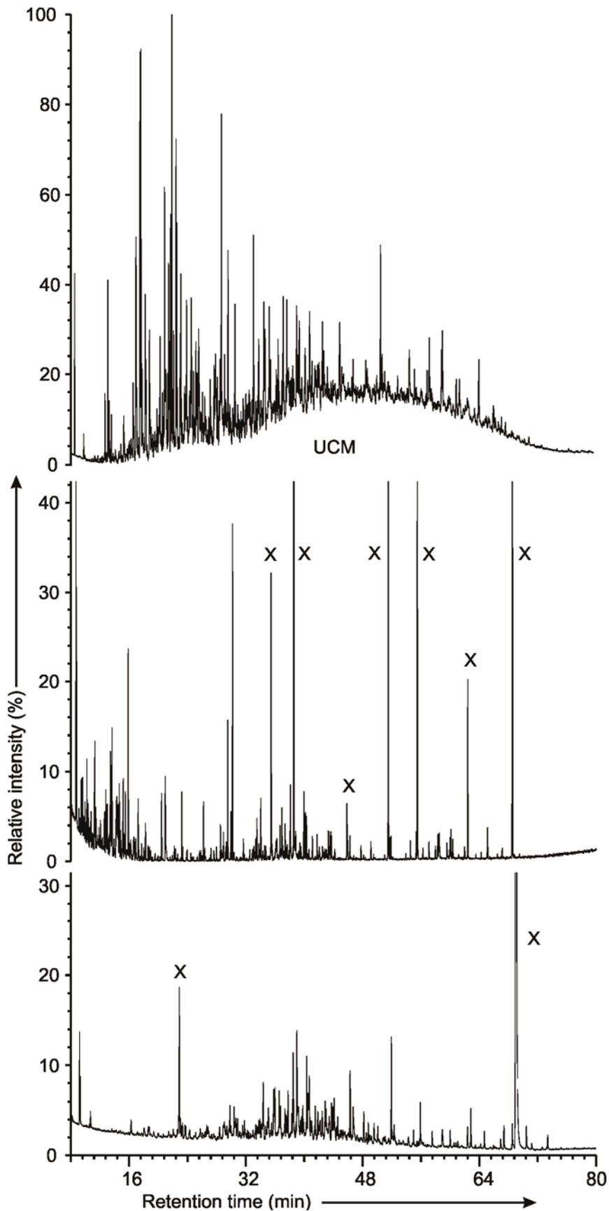
**Figure 7-1** Partial reconstructed ion current chromatograms of the degraded Monterey formation oil aromatic hydrocarbon fraction (top), an aqueous solution thereof (middle) and of the unpolar fraction of a tissue extract of mussels exposed to this aqueous solution (bottom). X denotes contaminants and artefacts as identified in Figure 3-6.
