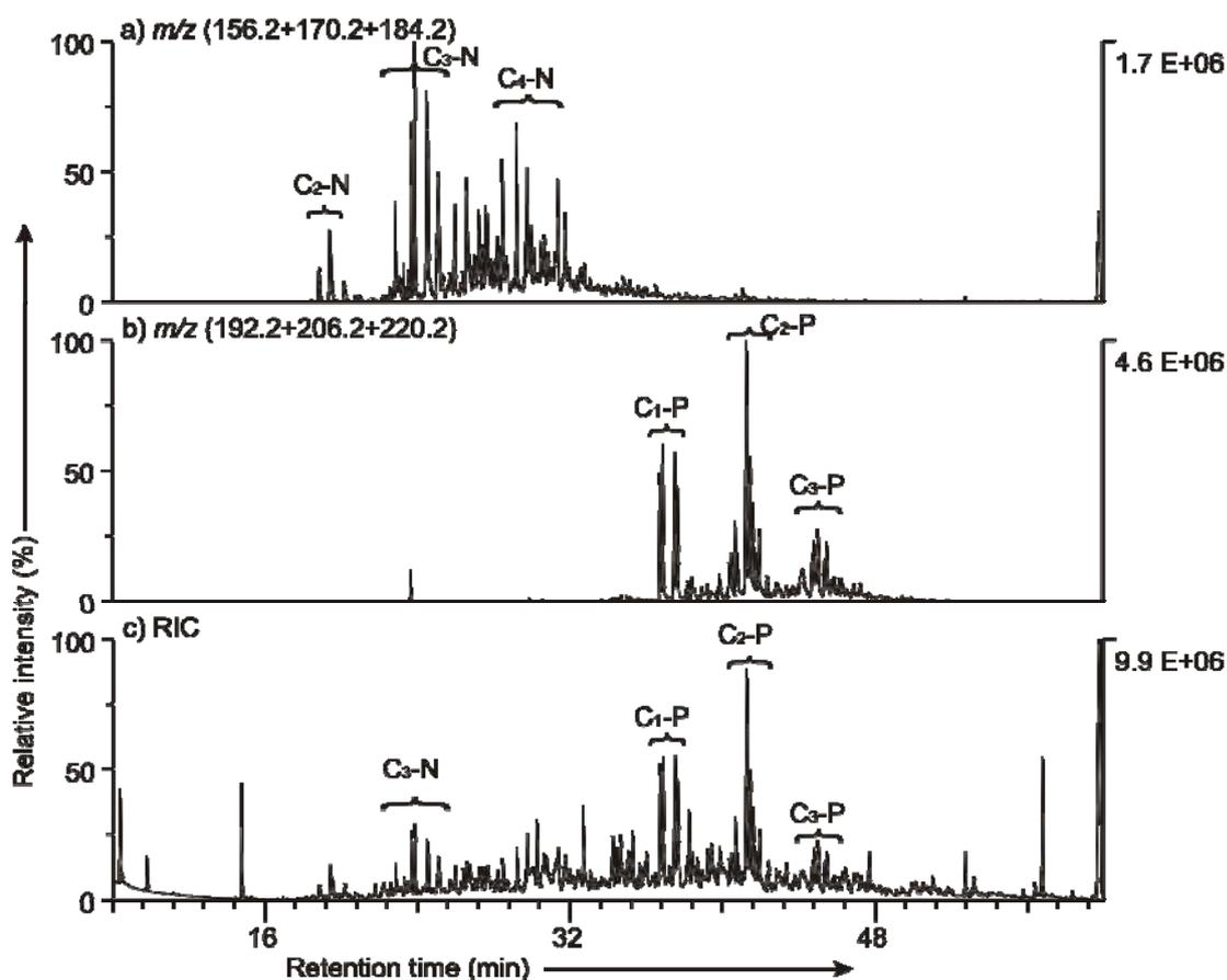
**Figure 6-4** Partial chromatograms of (a) molecular ions of  $C_2$ - to  $C_4$ -naphthalenes, (b) molecular ions of  $C_1$ - to  $C_3$ -phenanthrenes and (c) total ion current of accumulated compounds in sample Whv-I-uV-500; N = naphthalene, P = phenanthrene.
