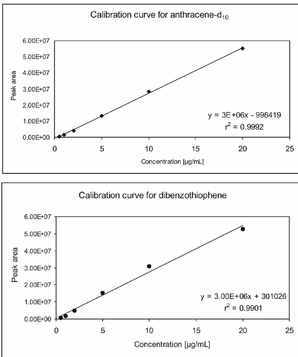
**Figure 3-5** Calibration curves for anthracene-d<sub>10</sub> (top) and dibenzothiophene (bottom) for GC-MS analysis, using  $m/z$  188.2 and  $m/z$  184.2, respectively.
