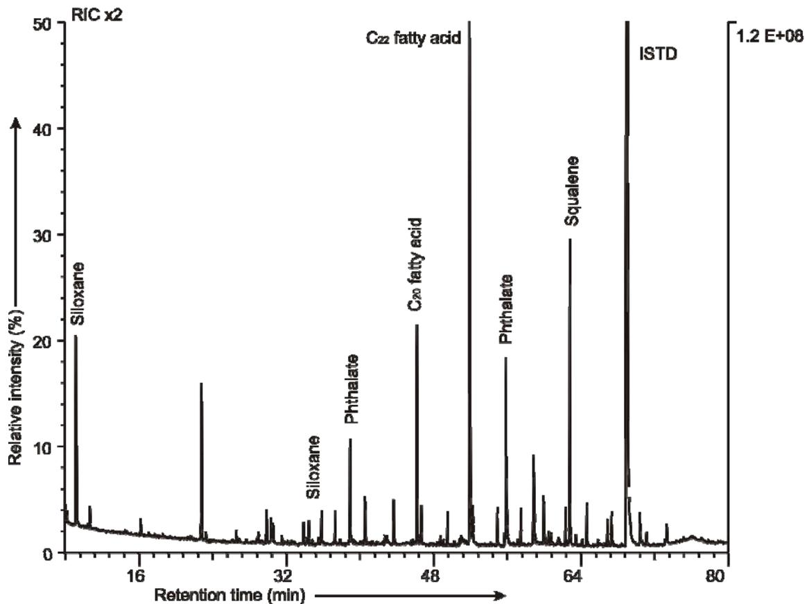
**Figure 3-6** Background compounds in partial reconstructed ion current chromatogram of the apolar fraction of a procedural blank, ISTD: internal standard tetradecyloctahydroanthracene
