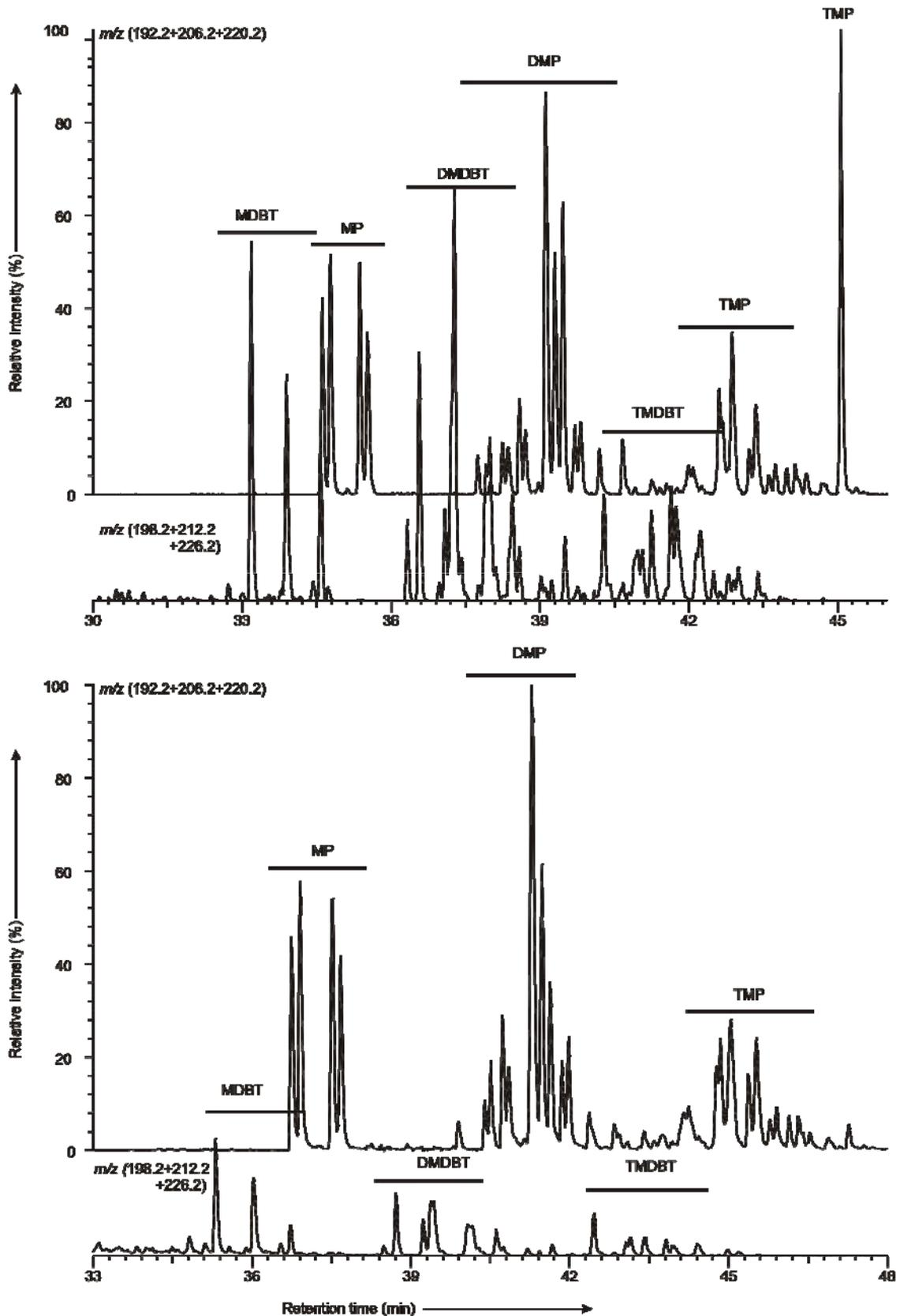
**Figure 6-6** Partial chromatograms of summed mass chromatograms of C<sub>1</sub>- to C<sub>3</sub>-phenanthrenes ( $m/z$  [192.2+206.2+220.2]) and C<sub>1</sub>- to C<sub>3</sub>-dibenzothiophenes ( $m/z$  [198.2+212.2+226.2]) in mussels exposed to the total aromatic hydrocarbon fractions of the undegraded Monterey Formation oil (sample Ply-uM-500, top) and of the undegraded Vienna basin oil (Whv-I-uV-500, bottom).
