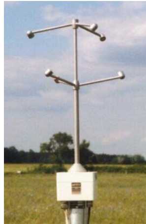
Figure 2.5: Photograph of a Metek ultrasonic anemometer.
