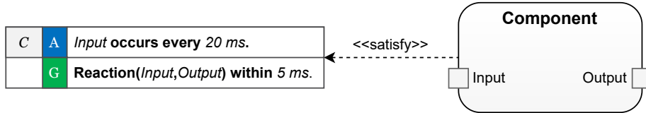
Fig. 2.1: Annotation of an A/G contract to a functional component
