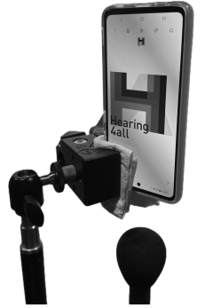
Figure B.1: Test setup of a smartphone calibration: A smartphone was placed on top of a calibrated microphone (microphone facing upwards). Frequency responses were recorded at several angles of incidence.
