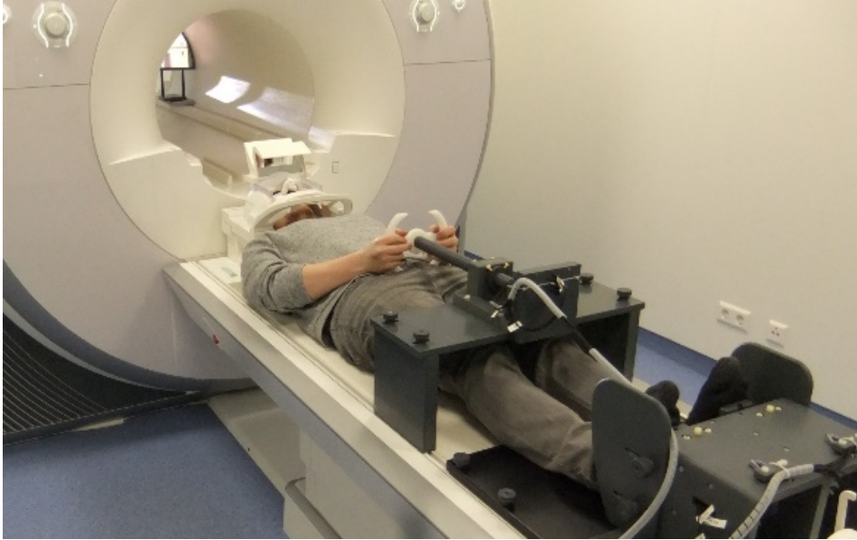
Figure 5.1. Setup of the MR compatible driving simulator
