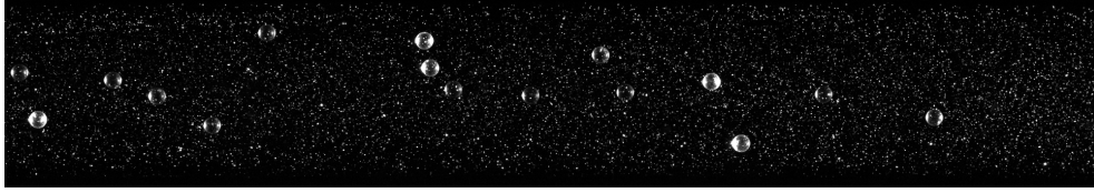
FIGURE 2.50: Snapshot of a tracer image with small polystyrene particles D_p = 0.1D , \phi_p \approx 0.5\% . Each particle has strong glare points due to the laser illumination from the right side.
