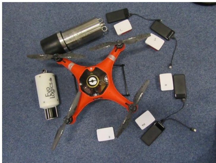
Figure 29: Overview of hardware components: The drone in the middle, five Raspberry Pis and two hydroacoustic modems (photograph by the author).
