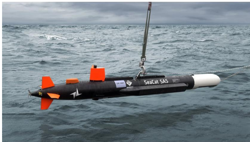
Figure 4: Image of the SeaCat UUV. This is a proprietary design by TKMS Atlas and is equipped with extensive sensor technology such as radar and communication systems for above-water and below-water operation (TKMS ATLAS ELEKTRONIK GmbH, SeaCat MK1, accessed 06.12.2025)
