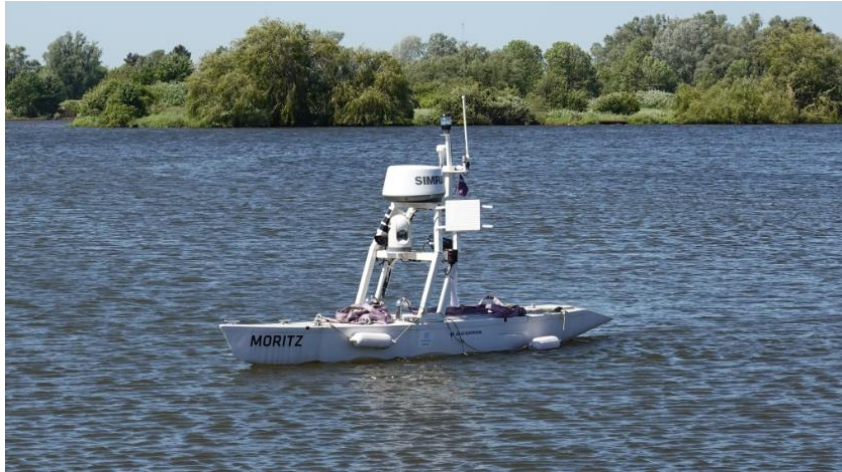
Figure 3: Picture of the USV “Moritz” in summer 2024. The USV is a proprietary design with extensive sensor technology and communication (radio & hydroacoustic), (photograph by the author).
