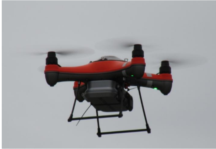
Figure 28: Overview of the drone used with a Raspberry Pi as a Relay Node (photograph by the author).
