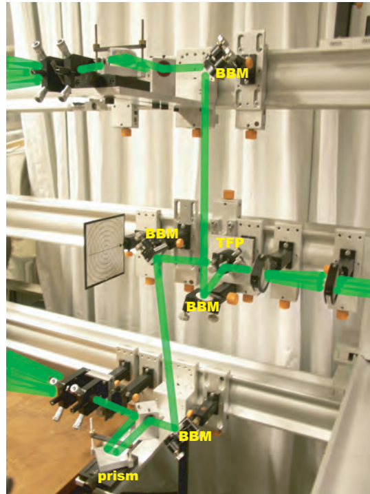
Figure 6.3: Photograph of the RBDU equipped with optional tools for fine-adjustment of the reference beams path-lengths and beam expansion with spatial frequency filter (beam propagation artificially added for clarity).
