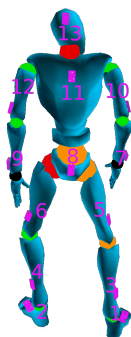
Figure 7.1: Placement of the 13 CAPTIV IMU sensors on major joints of a participant.
