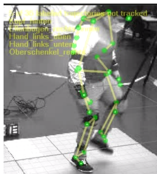
Figure 7.2: Visualization of detected reflective markers in the Qualisys System
