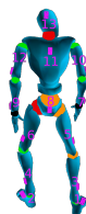
Figure 8.1: Placement of the 13 CAPTIV IMU sensors on major joints of a participant.
