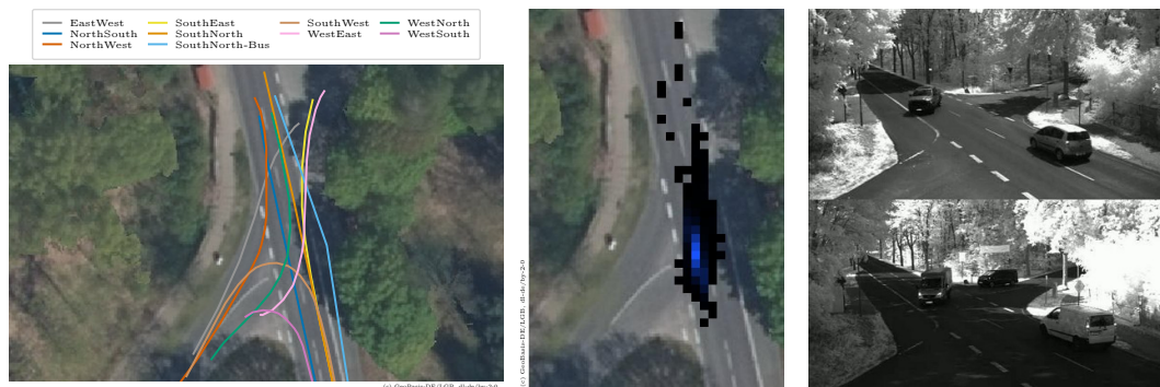
Figure 6.31: Left: The routes of the measurement site. Middle: The distribution of crossing points on the measurement site for the north-west scenario. Right: Examples of breaking traffic participants in crossing scenarios on the federal road. [144]
