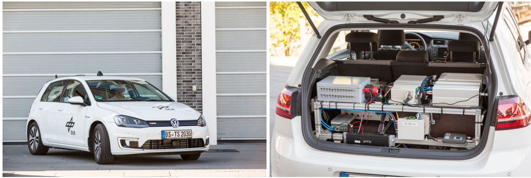
Figure 6.22: The FASCar of the DLR (left panel) as a reference vehicle for qualitative analysis of test beds using TASI, with the measurement system located in the trunk of the FASCar (right panel). © DLR
