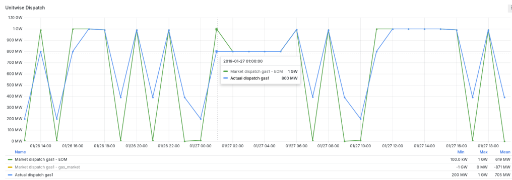
Figure 5.16: Visualization of hourly market dispatch and actual feasible dispatch using clearing mechanism and bidding strategies described in Section 4.3.1 for the fuel market scenario. The tooltip shows a deviation due to a ramping constraint, which the market did not respect, leading to a reduced dispatch.
