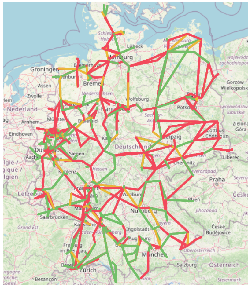
Figure 5.6: Visualization of simulation grid from a given PyPSA input dataset. Utilization of grid lines is visualized from power flow calculation in market results (green – low utilization; yellow – medium utilization; red – high utilization).
