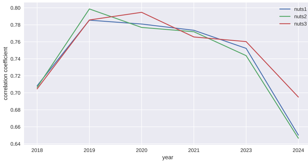
Figure 5.10: Summary of correlation coefficient with historical benchmark dataset of ENTSO-E between market simulation with different NUTS aggregations. One can see that the focus on correct price modeling and bidding behavior has a higher influence on the results than the aggregation, while all simulations provide good out-of-the-box results.
