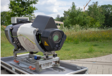
Figure 2.3: The SpinnerLidar along with its mounting mechanism at the University of Oldenburg.
