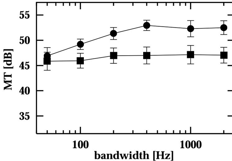
Figure 5.10: *Simulated data for a 2kHz sinusoidal signal in random noise (circles) and comodulated noise (squares). In this simulation instead of a gammatone filter a rectangular filter with the same bandwidth was applied.*
