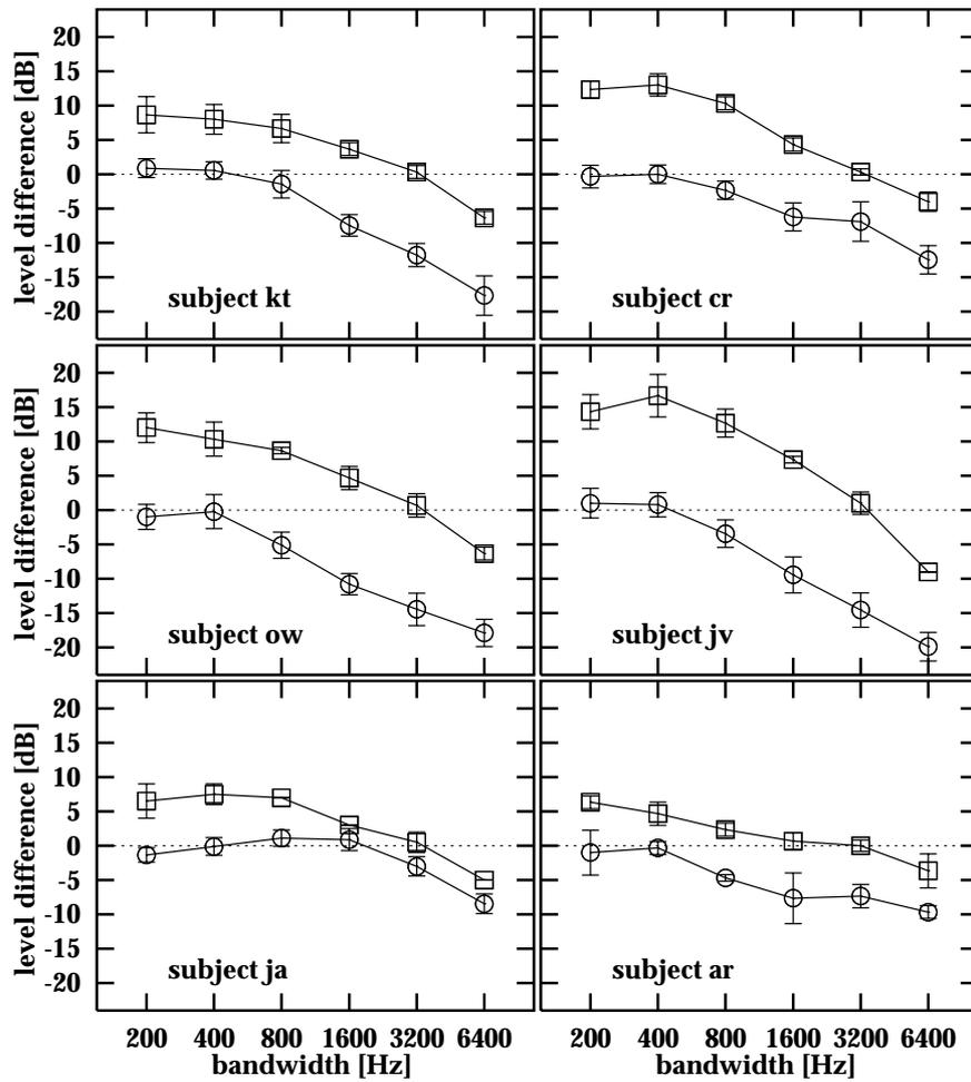
Figure 2.4: Equal-loudness levels measured with interleaved tracks as function of test-signal bandwidth from six listeners. Signal duration was 1000 ms. Two reference bandwidth were tested: 400 Hz (○), and 3200 Hz (□). The vertical bars show plus and minus one standard deviation of the mean.
