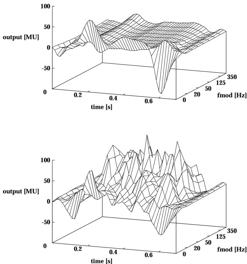
Figure 4.8: *Internal representation of the test signal calculated as the difference between the actual internal representation of the test signal plus masker and the stored mean internal representation of the masker alone. The upper panel shows the internal representation of a test signal with a bandwidth of 4 Hz, in the lower panel the test-signal bandwidth was 256 Hz. In both conditions the masker bandwidth was 4 Hz and the test-signal level was 15 dB above the masker level of 70 dB SPL.*
