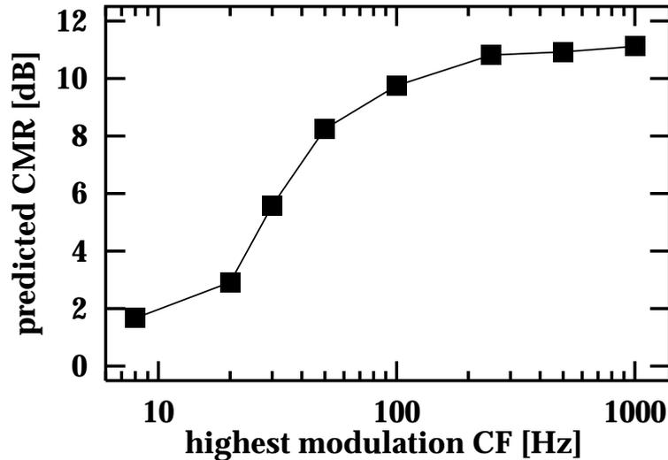
Figure 5.9: Simulated CMR for a masker bandwidth of 1000 Hz, a modulator bandwidth of 50 Hz, and a signal frequency of 2 kHz. Parameter is the highest modulation center frequency of the modulation filters.
