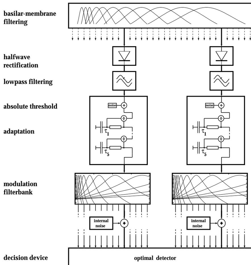
Figure 4.1: Block diagram of the psychoacoustical model as described in Dau et al. (1997a+b). The signals are preprocessed with a gammatone filterbank, subjected to adaptation and filtered by a modulation filterbank in each peripheral filter. Finally an internal noise is added. The decision device is realized as an optimal detector.
