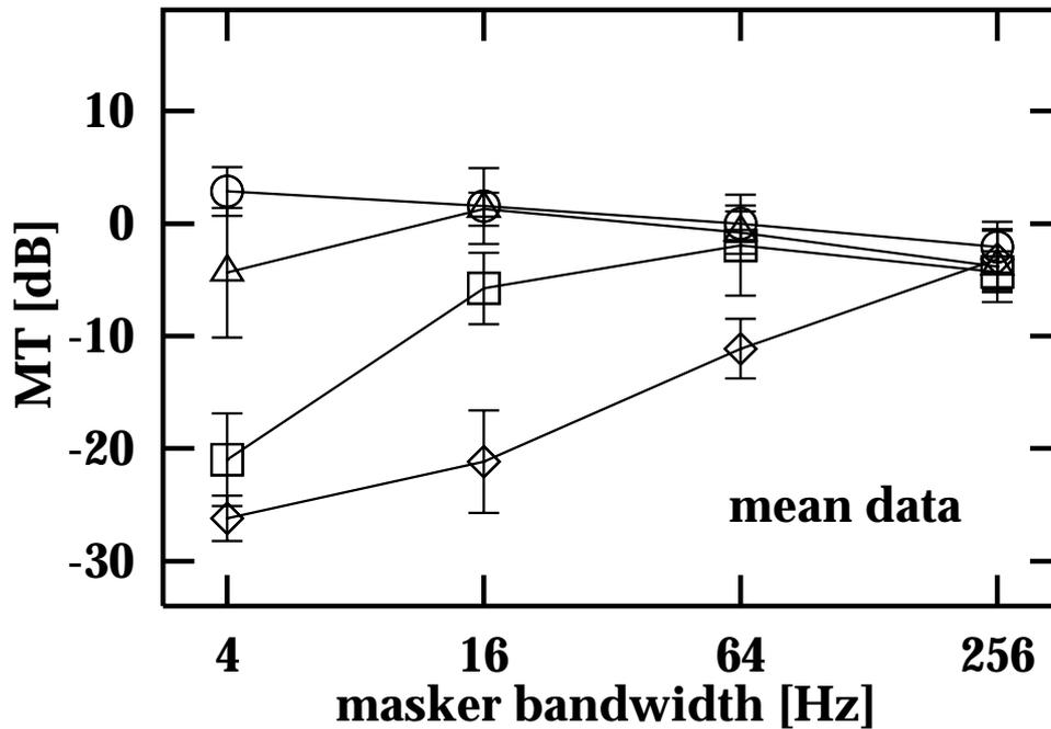
Figure 4.6: Mean measured data over four subjects for a bandpass-noise signal masked by a bandpass-noise masker as a function of the masker bandwidth. Symbols are the same as in Fig. 4.5.
