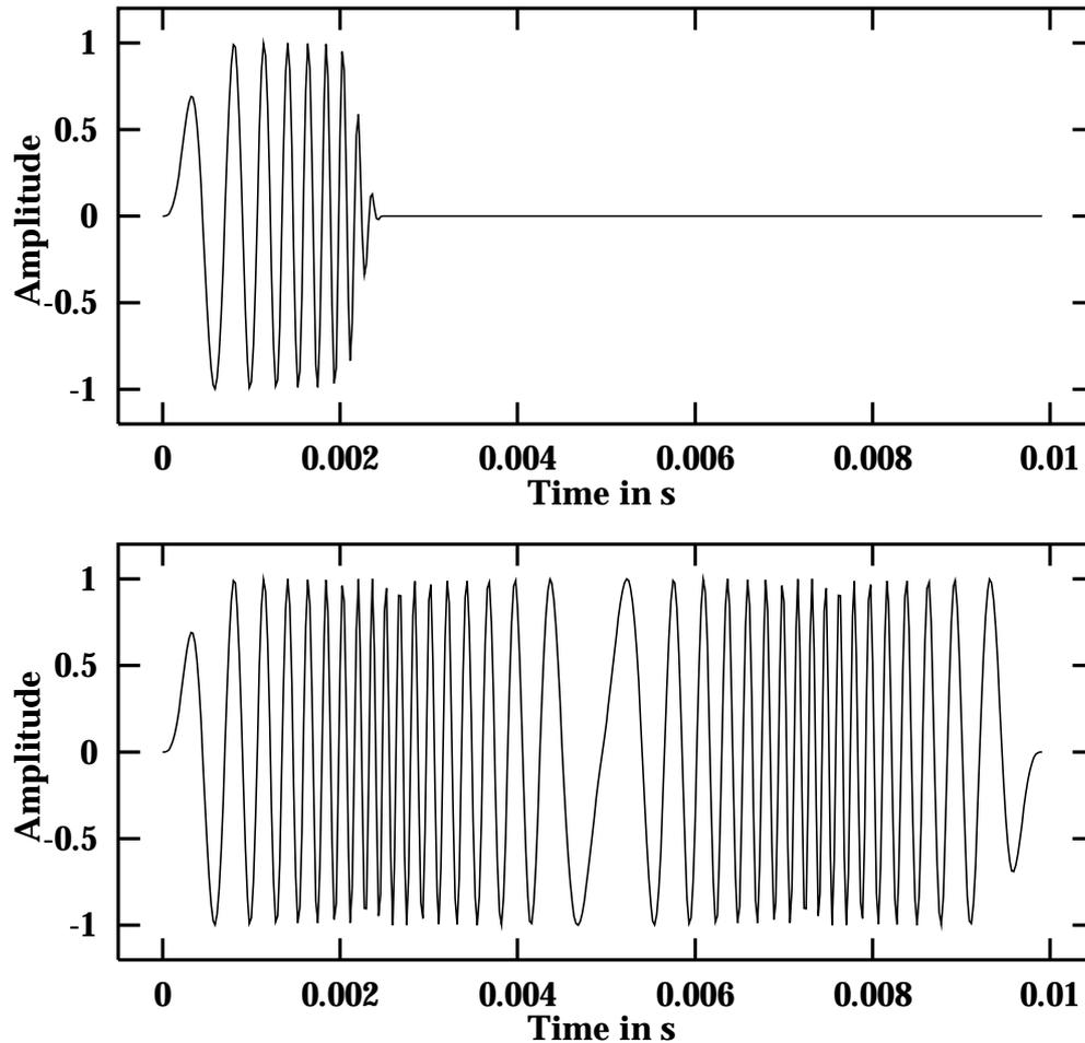
Figure 3.3: *Time signals for chirp stimuli with a bandwidth of 6400 Hz and a duration of 2.5 msec (upper panel) and 10 msec (lower panel), respectively.*
