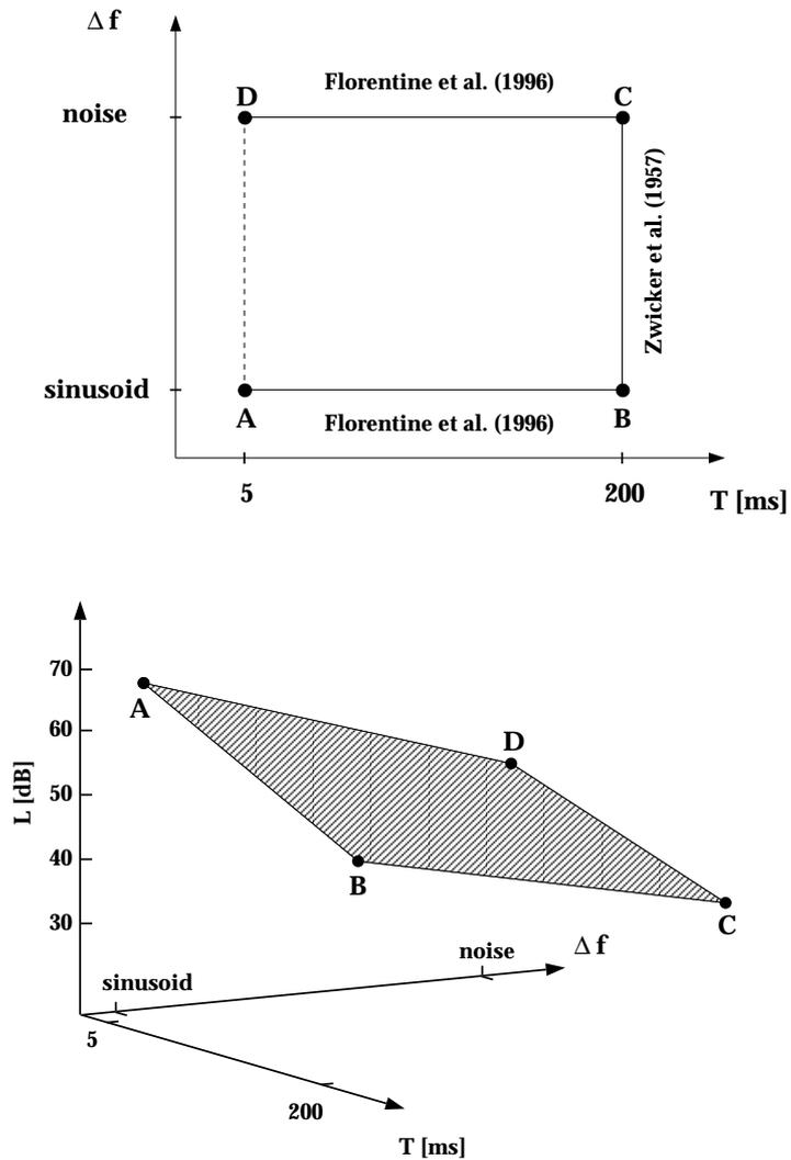
Figure A.1: *Upper panel: Illustration for deriving loudness summation for short signals from experimental results on temporal integration of loudness and loudness summation for stationary signals. Lower panel: Equal loudness level surface for a 5-msec white-noise signal with a level of 50-dB SPL.*
