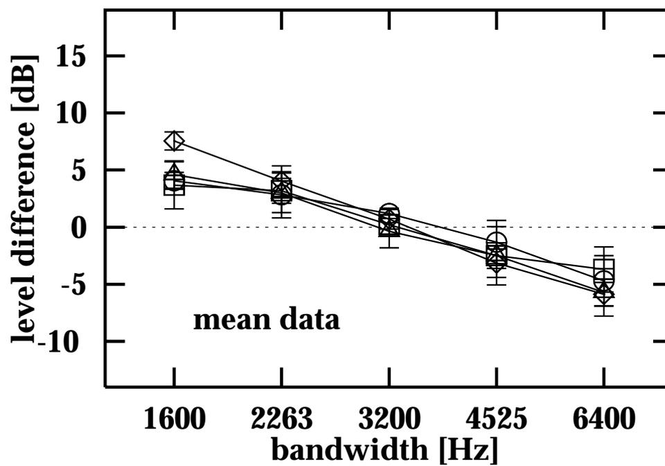
Figure 3.5: Averaged loudness summation for chirp trains from six listeners. Signal duration was either 2.5 msec (circles), 5 msec (squares), 10 msec (triangles), or 400 ms (diamonds). The level difference between the level of test and reference signal needed to obtain equal loudness are plotted as Figure 3.4. The vertical bars show plus and minus one interindividual standard deviation of the mean.
