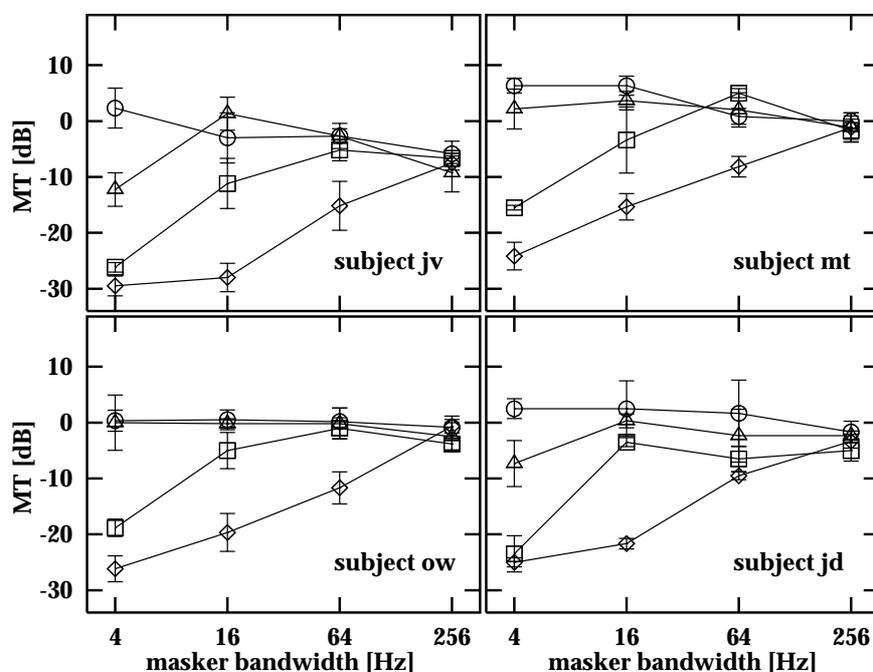
Figure 4.5: Masked threshold ( $MT$ ) of a bandpass-noise signal masked by a bandpass-noise masker as a function of masker bandwidth. Parameter is the test-signal bandwidth: 4 Hz ( $\circ$ ), 16 Hz ( $\triangle$ ), 64 Hz ( $\square$ ) and 256 Hz ( $\diamond$ ). Individual data are shown for four normal hearing subjects.
