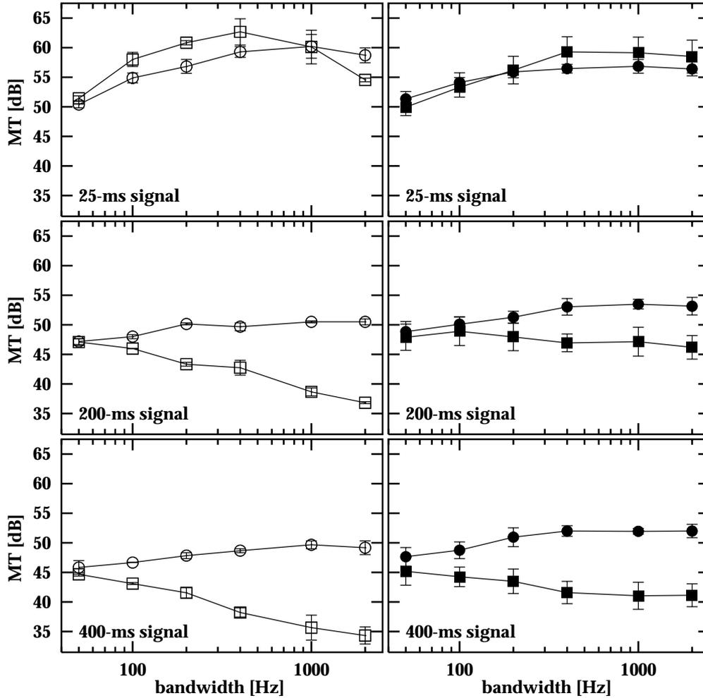
Figure 5.5: Mean measured thresholds over three subjects (left row of panels) and simulated thresholds (right row of panels) for a signal presented in random noise ( $\circ$ ) and modulated noise (modulator bandwidth of 12.5 Hz,  $\square$ ) as a function of the masker bandwidth. Signal duration was either 400 (upper panels), 200 (middle panels), or 25 ms (lower panels). The signal frequency was 2 kHz.
