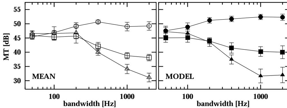
Figure 5.8: Mean data over three subjects (right panel) and simulated data (left panel) showing thresholds for a signal presented in random noise ( $\circ$ ), in modulated noise with a 50 Hz lowpass-noise modulator ( $\square$ ), and in modulated noise with a 50 Hz square-wave modulator ( $\triangle$ ) as a function masker bandwidth.
