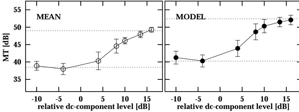
Figure 5.7: Mean measured data (right panel) and simulated data (left panel) for a sinusoidal signal in the presence of a 1000 Hz modulated band-pass noise-masker as a function of the added dc-component to the modulator. In addition thresholds for random noise (upper line) and modulated noise (lower line), where no dc-value is added (experimental condition as in Fig. 1) are shown.
