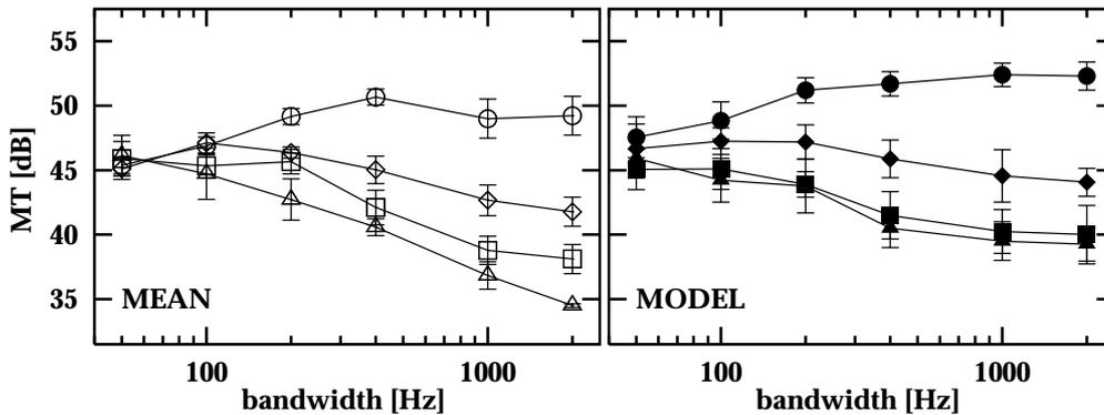
Figure 5.4: Mean measured data over three subjects (left panel) and simulated thresholds (right panel) for a signal presented in random noise ( $\circ$ ) and modulated noise as a function of the masker bandwidth. The modulator bandwidth was 12.5 Hz ( $\triangle$ ), 50 Hz ( $\square$ ), and 200 Hz ( $\diamond$ ), respectively.
