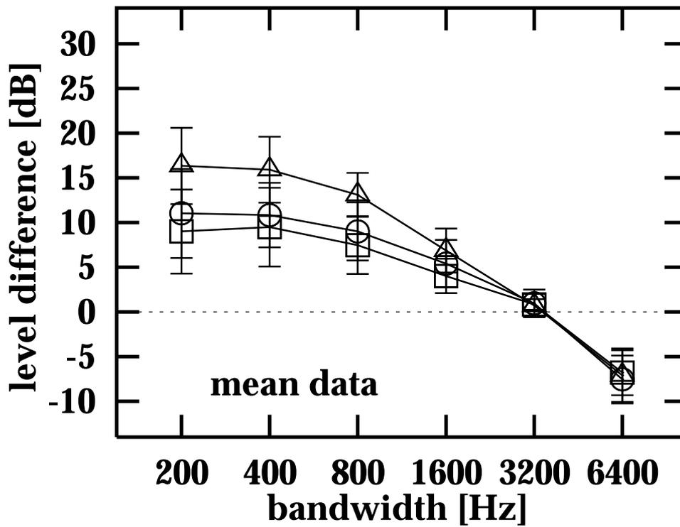
Figure 3.2: Averaged loudness summation for bandpass-noise signals from ten listeners. Signal duration was either 1000 msec (squares), 100 msec (circles), or 10 msec (triangles). The level differences between the level of test and reference signal needed to obtain equal loudness are plotted in the same manner as Figure 3.1. The vertical bars show plus and minus one interindividual standard deviation from the mean.
