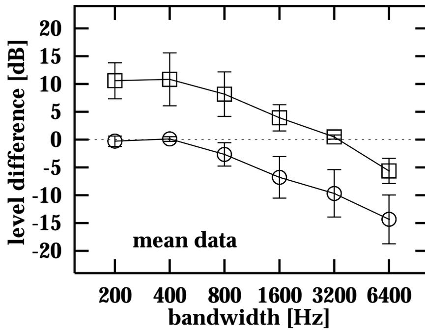
Figure 2.5: Averaged equal-loudness levels measured with interleaved tracks as function of test-signal bandwidth for two reference bandwidths from six listeners. Symbols are the same as in Fig. 2.4. The vertical bars show plus and minus one standard deviation of the means across the six subjects.
