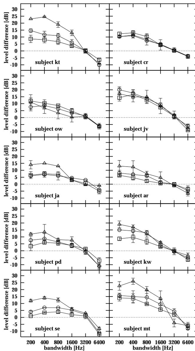
Figure 3.1: Loudness summation for bandpass-noise signals from ten listeners. Signal duration was either 1000 msec (squares), 100 msec (circles), or 10 msec (triangles). The level differences between the level of test and reference signal needed to obtain equal loudness are plotted as a function of the bandwidth of the test signal. The vertical bars show plus and minus one standard deviation of the mean.
