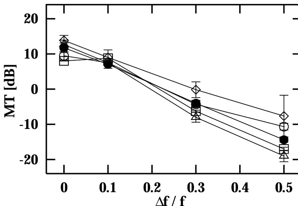
Figure 4.2: Masked thresholds ( $MT$ ) for a sinusoidal signal presented in notched noise as a function of masker bandwidth. The signal frequency was 1 kHz. Open symbols indicate measured thresholds (JA (○), PH (◇), TD (□) JV (△)). Closed symbols indicate simulated thresholds.
