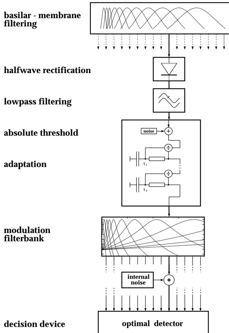
Figure 5.1: Block diagram of the psychoacoustical model as described in Dau et al. (1997a). The signals are preprocessed, subjected to adaptation, filtered by a modulation filterbank and finally added to internal noise. The decision device is realized as an optimal detector.
