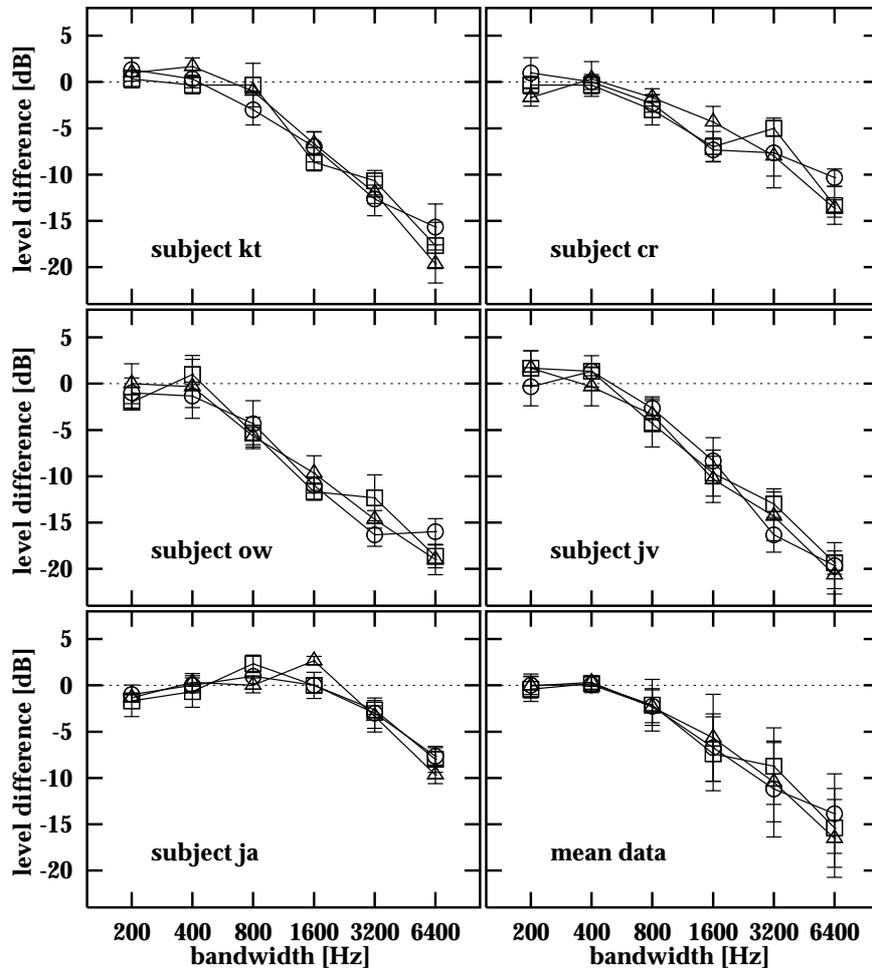
Figure 2.3: Equal-loudness levels measured with interleaved tracks as function of test-signal bandwidth. The level differences needed to obtain equal loudness between test and reference signal are plotted in the same way as in Fig. 2.1. Signal duration was 1000 ms. The reference was the same as in the previous figures.
