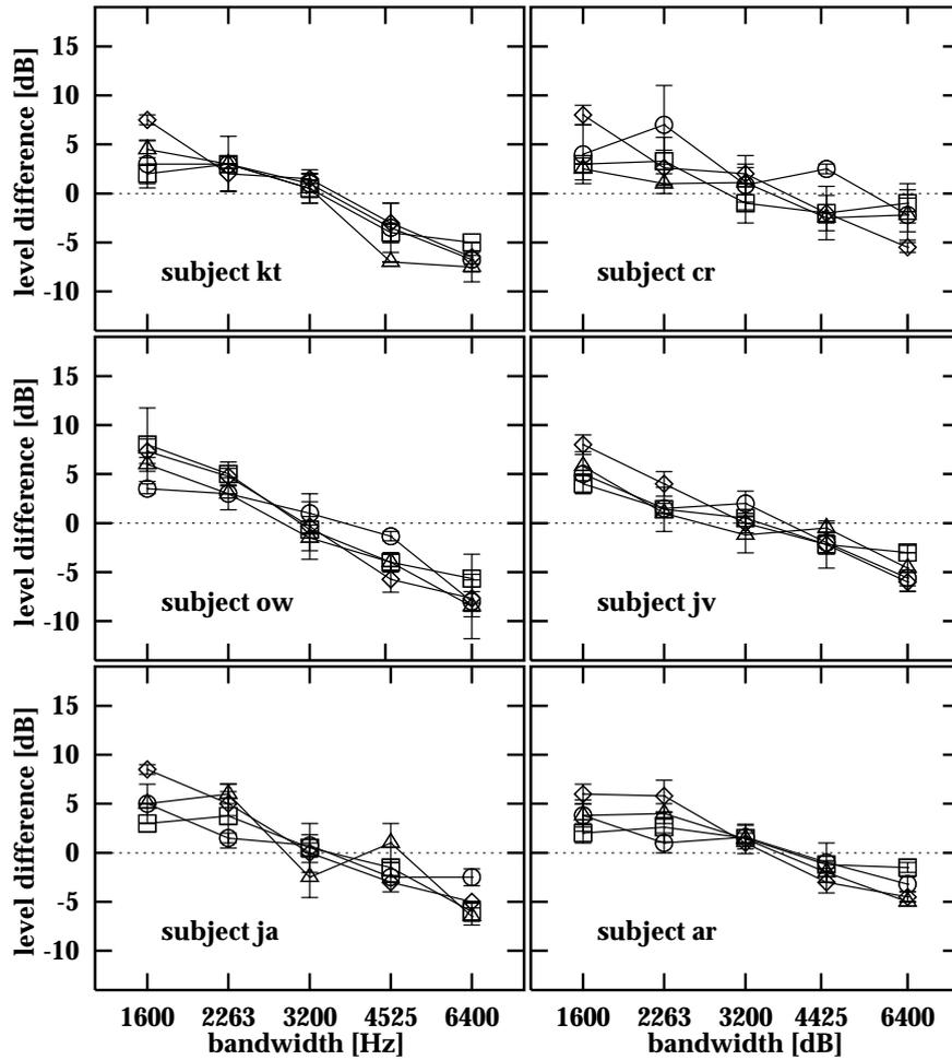
Figure 3.4: Loudness summation for chirp trains from six listeners. Signal duration was either 2.5 msec (circles), 5 msec (squares), 10 msec (triangles), or 400 ms (diamonds). The level differences between test and reference signal needed to obtain equal loudness are plotted as a function of the bandwidth of the test signal. The vertical bars show plus and minus one standard deviation of the mean.
