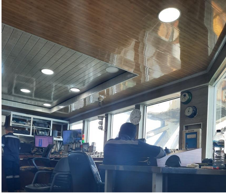
Figure 26: Mining navigation room (Personal documentation, 2022). Details: the navigation room is where the head of the mining ship navigates the ship, instructs mining workers using microphones, and operates the cutter suction dredger.
