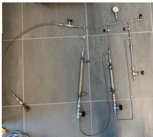
Figure 21: Theoretical setup for the solvation and precipitation with CO 2 .
