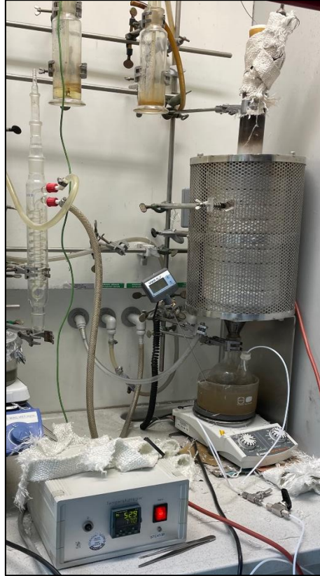
Figure 7: Steam activation oven for ST treatment of PL
