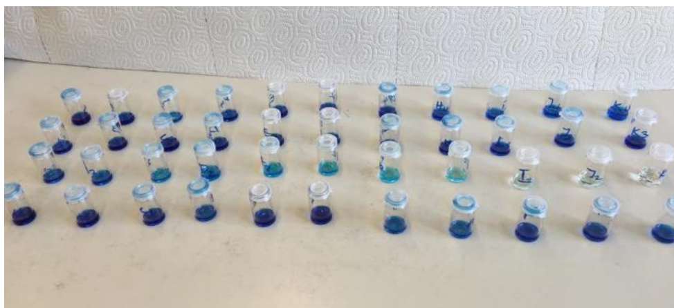
Figure 19: Methylene-blue dye Absorption Experiment
