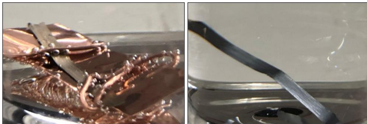
Figure S9: Dealloying of Zn 80 Cu 20 alloy ribbons in 1.3 M NaOH, showing hydrogen bubble formation on the Cu substrate (left image) and the absence of hydrogen bubbles on the pure ribbon surface without Cu attached (right image). Figure reprinted with permission from ref. 52.
