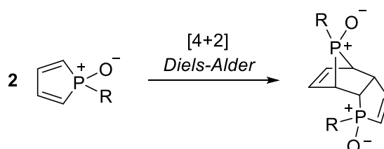
Scheme 35 – Exemplaric [4+2] Diels-Alder cycloaddition of a phosphole oxide, typically giving the endo dimer. [137, 139]
