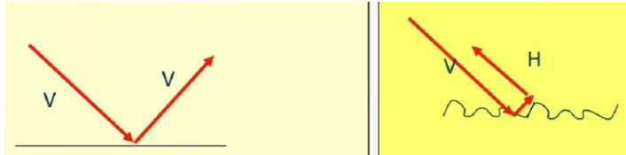
Figure 2.19: Scattering and surface structure [94].
