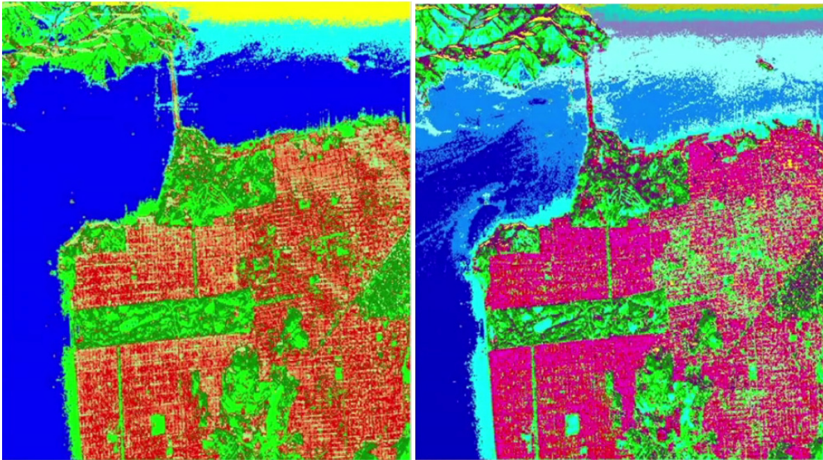
(a) H-\bar{\alpha} Wishart classification (four iterations). (b) H-A-\bar{\alpha} Wishart classification (four iterations).
