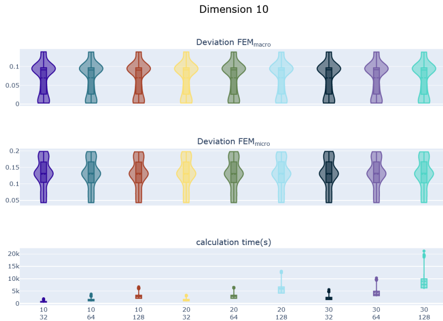
Fig. B.14.: Violin plots showing the impact of the the number of samples for local FLA and the number of repetitions of the local FLA on the deviation of FEM from centrally computed counterpart for dimension 10.
