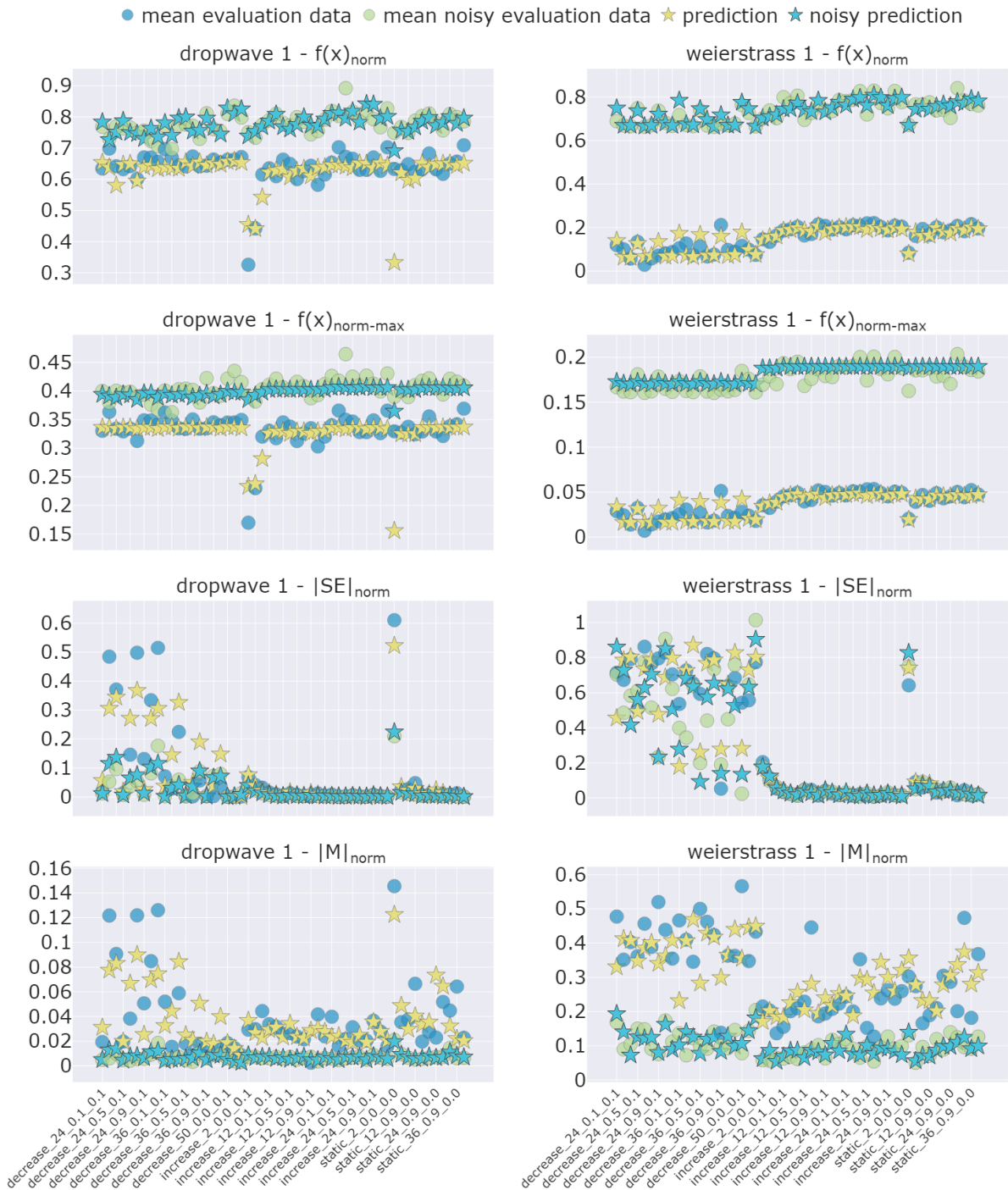
Fig. 6.20.: Predictions for noiseless and noisy evaluation data after retraining with a mixed set of training data. The corresponding metric is always plotted on the y-axis. The CTVs are plotted on the x-axis and are encoded in the form mode\_k\_p\_α .
