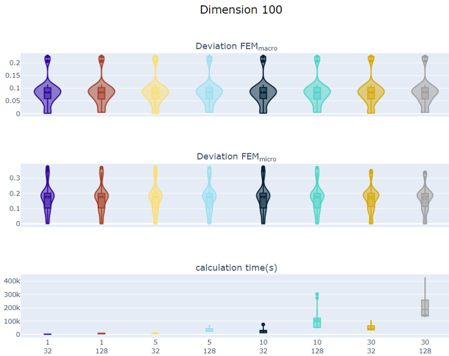
Fig. B.15.: Violin plots showing the impact of the the number of samples for local FLA and the number of repetitions of the local FLA on the deviation of FEM from centrally computed counterpart for dimension 100.
