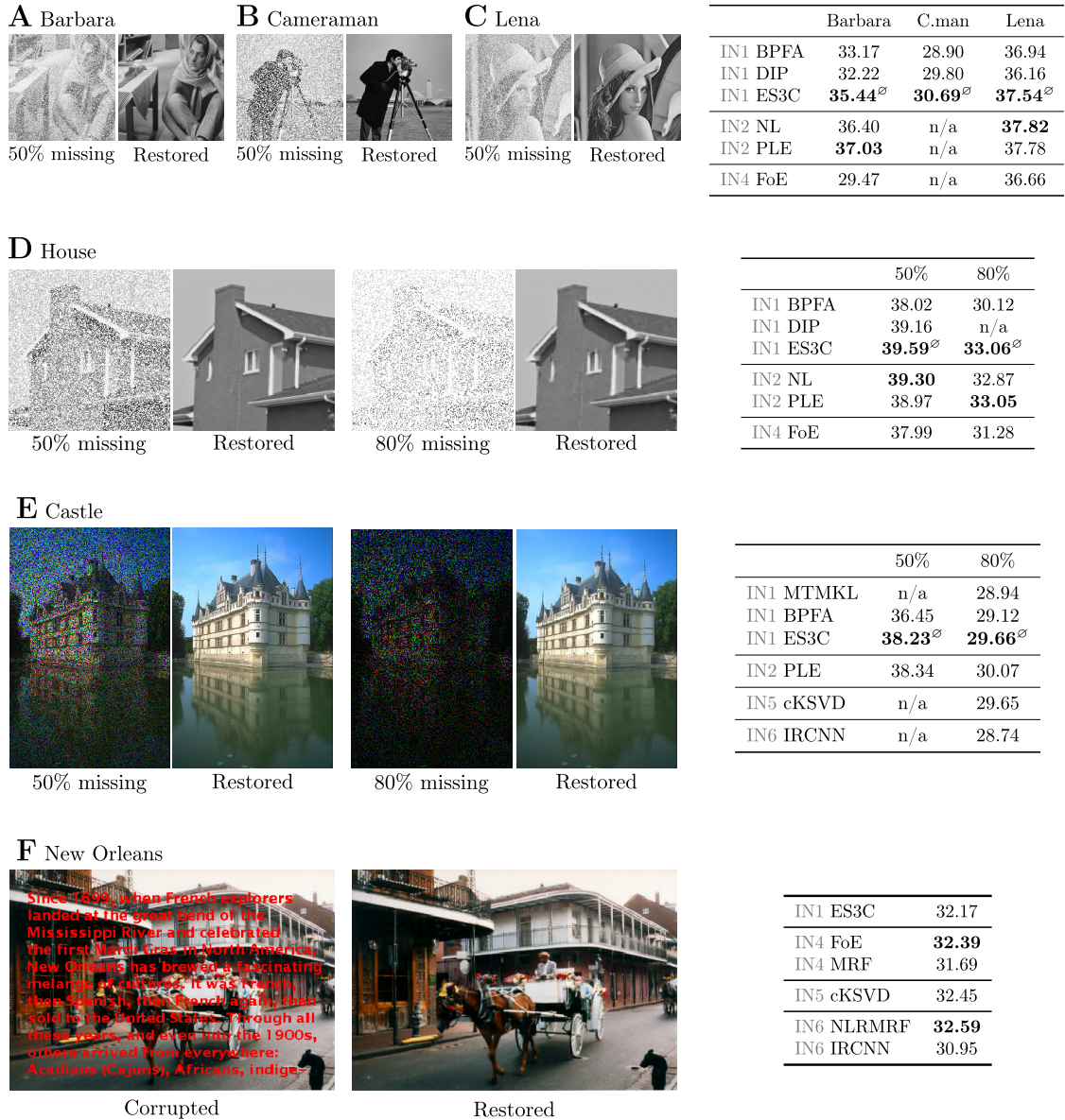
Figure 2.7: Inpainting results for “Barbara”, “Cameraman”, “Lena”, “House”, “Castle” and “New Orleans”. For the performance comparison, different approaches are grouped and labeled according to Tab. 2.2. In each group the highest PSNR value is marked bold. Numbers marked with ⊘ in A to E correspond to averages over multiple independent runs of the experiment using different realizations of missing values (see text for details; the performance of ES3C in the individual runs is reported in Tab. 2.S1 in Sec. 2.S6). On the left, we illustrate the reconstructed images obtained with ES3C in the run with the highest PSNR value.
