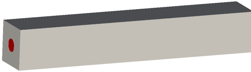
Figure 4.12: Shape of the domain with the turbulent inlet patch in red.
