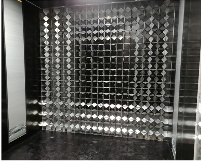
Figure 4.1: Active grid installed in the closed test section.
