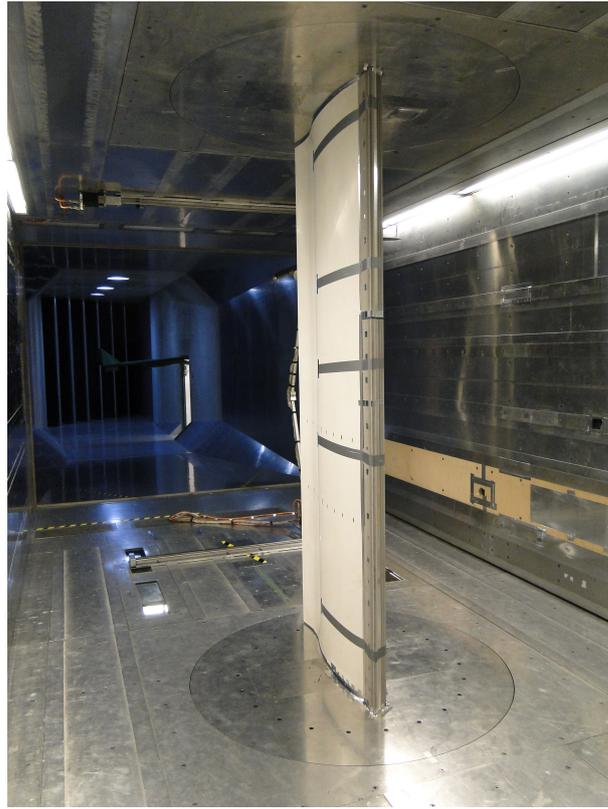
Figure 4.2: The wind tunnel setup of testing profile 1 in open section wind tunnel at the German-Dutch wind tunnels
