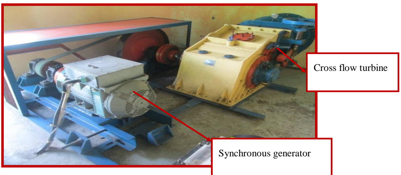
Figure 27: Cross flow turbine with synchronous generator
