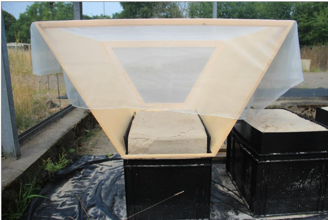
Fig. 3.4: Photo of the wind tunnel installed on an artificial bare dune with the upper 10 cm of soil exposed.
