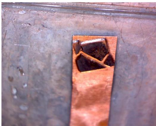
**Figure 25:** Broken Si electrode after the experiment.
