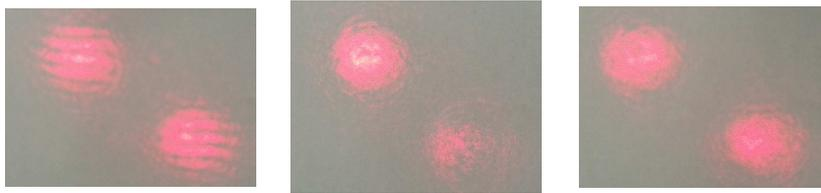
Figure 3.10: Beam profiles of the LDI at the plane of the photodiodes. They are displayed on a white screen for adjustment. Left: bad adjustment. Middle: good adjustment. Right: working position
