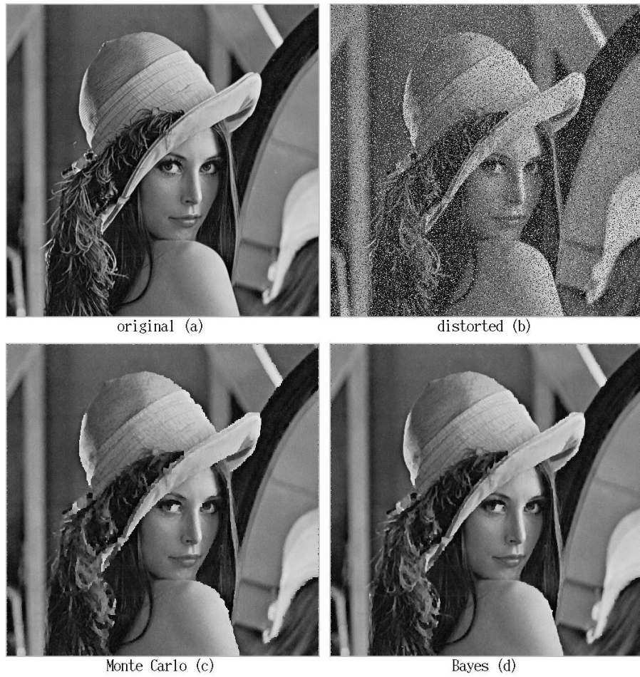
Figure 6.5: Grey-level image (256 states, 8 bit) distorted by random noise with a probability of p = 0.3 . The displayed images are: (a) original, (b) distorted (rms=48.51), (c) Monte Carlo snapshot (rms=11.83) and (d) Bayes estimate (rms=9.01) after 750 steps.
