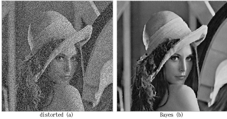
Figure 6.10: Image distorted by random noise with p = 0.45 ( rms=59.27 ) (a). The Bayes restoration ( rms=10.6 ) (b) is obtained after 750 steps. The information loss due to noise is close to the information contained in the prior.
