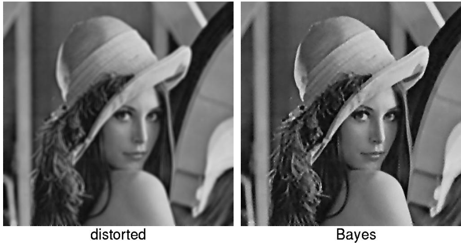
Figure 6.20: Example of deblurring. The left image shows the effect of applying a pill-box blur filter of size 7x7 pixels. The right image shows the restoration.
