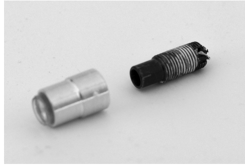
Figure 5.3: Photo of the CAW100 collimator lens inside the custom made lens holder (silver) and custom made laser diode mount (black) with precision thread to adjust the focus.
