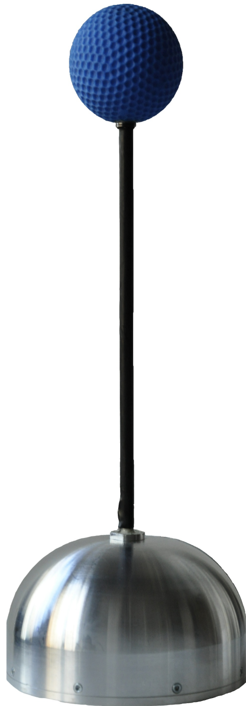
Figure 5.14: Improved sphere anemometer with impermeable, dome-shaped aluminum housing. The coarsely dimpled sphere with surface filling pattern is attached to the GFP tube. The supply cables for the laser are fixed to the downstream side of the tube and covered with a shrinking hose to reduce oscillations.
