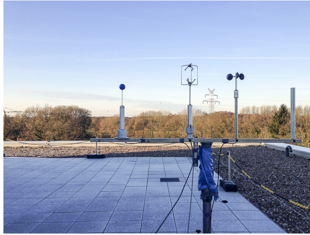
Figure 9.6: Photo of the anemometer boom with sphere, sonic and cup anemometer (left to right) installed on the roof top of the WindLab building. View from 0^\circ wind direction (south-east).
