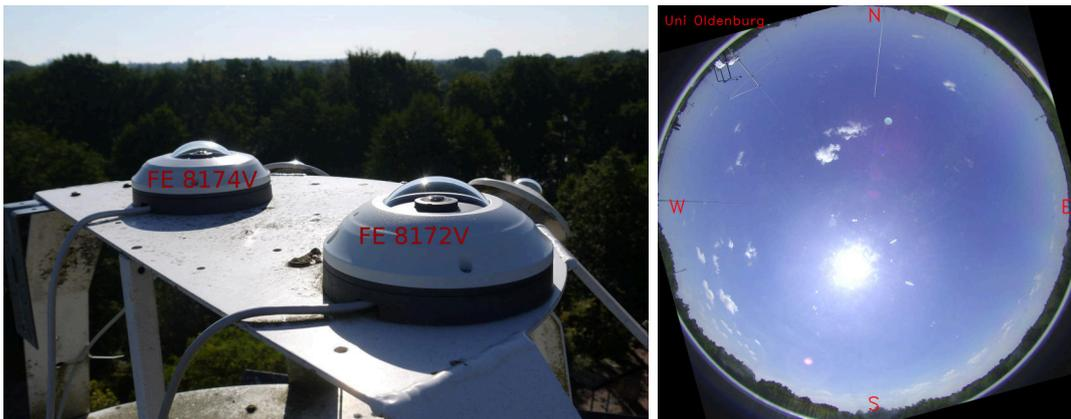
**Figure 3.2:** Left: Sky imagers at the University of Oldenburg. Right: Example image of the *Vivotek FE8172V* camera. The image has been rotated to point northwards at the top.
