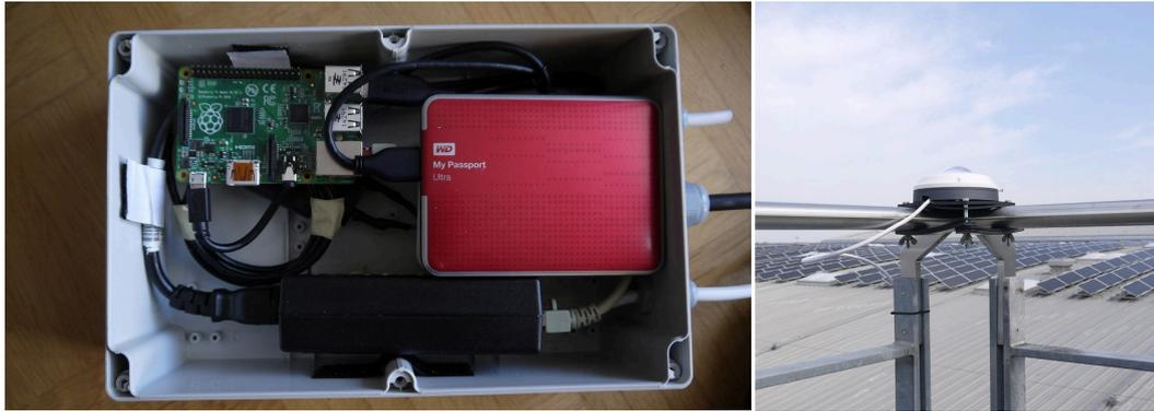
**Figure 3.4:** Weather resistant junction box with the Raspberry Pi, the external storage and the power-over-ethernet (POE) adapter used for the experiment (image left). The image in the right shows the camera mounted on the rooftop (PV plant in the background).
