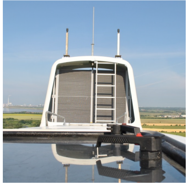
Figure 5-2: Downwind view on the experimental turbine with two ultrasonic acoustic resonance wind speed and direction sensors mounted on top of the cooler.
