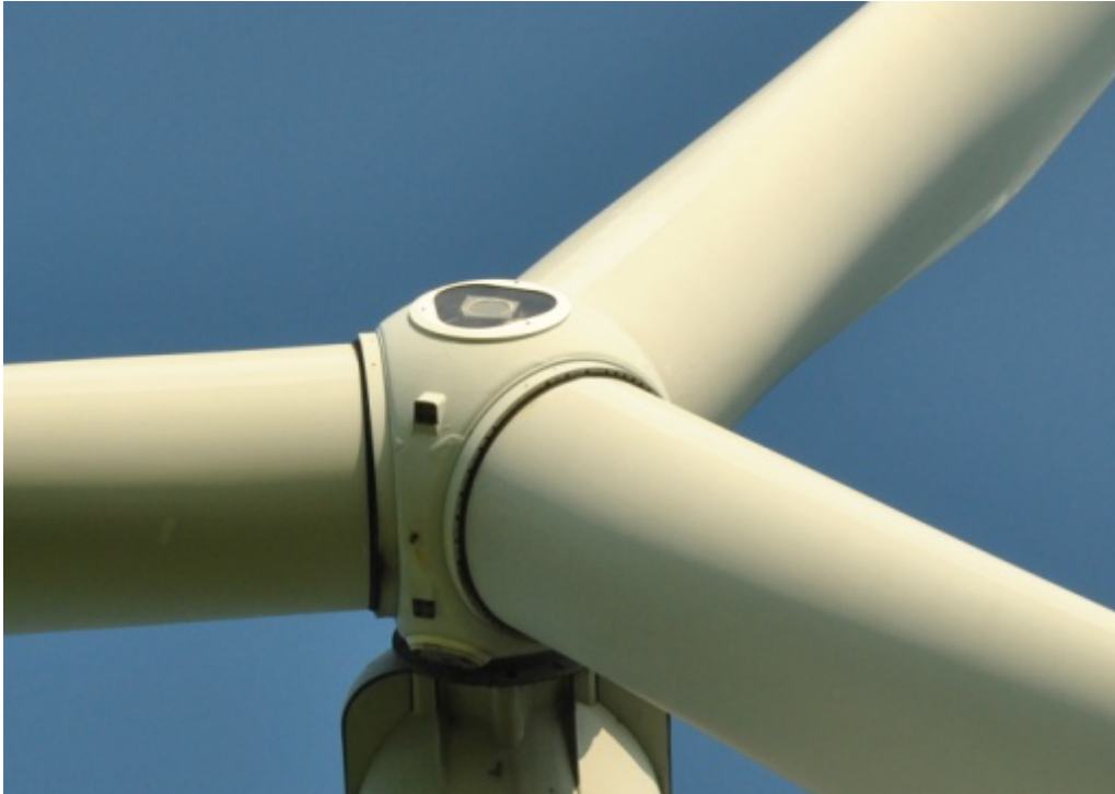
Figure 1-4: NEG Micon NM80 wind turbine (today Vestas) equipped with a lidar in the rotating hub. Setup and experiments are presented in Chapter 5.
