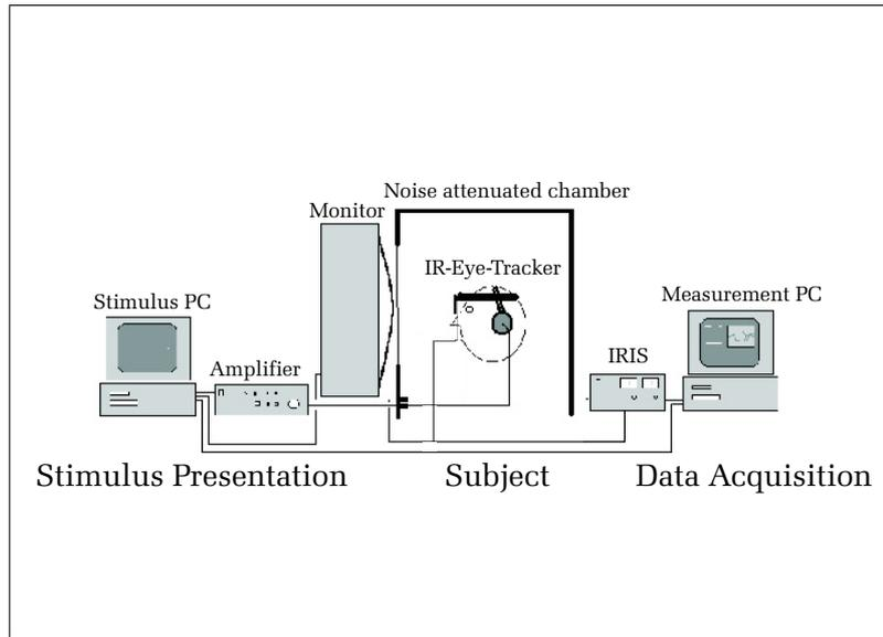
Figure 2.1: Schematic diagram of the apparatus used in all experiments.
