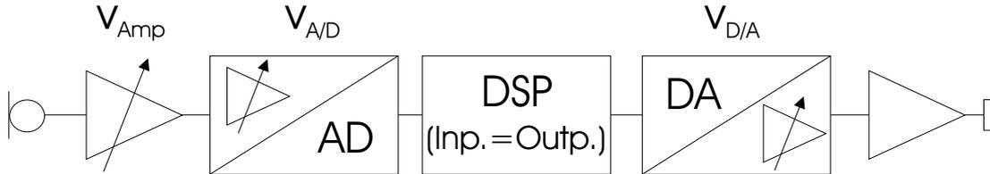
**Figure 2.3:** Block diagram of signal flow in the DASI-2 [Raß and Steeger, 2000].
