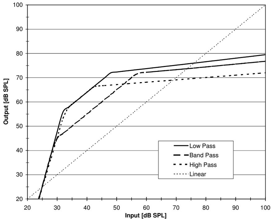
**Figure 2.4:** Example of an actually implemented I/O-characteristics for algorithm AV in the three frequency channels adjusted for one test subject (MW, right ear). The I/O-characteristics for the low- and high-pass channel had to be limited to a maximum of 24 dB (maximum possible gain given by the implementation of the gain Table). The maximum gain of the band pass signal had to be further reduced to avoid feedback.
