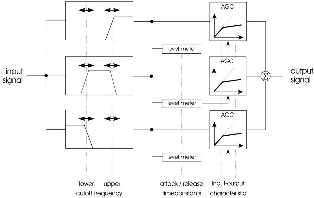
**Figure 2.1:** Schematic overview of the 3-channel dynamic compression master-hearing-aid.
