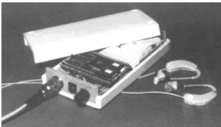
**Figure A.1:** *The wearable hearing-aid device (DASi-2).*
