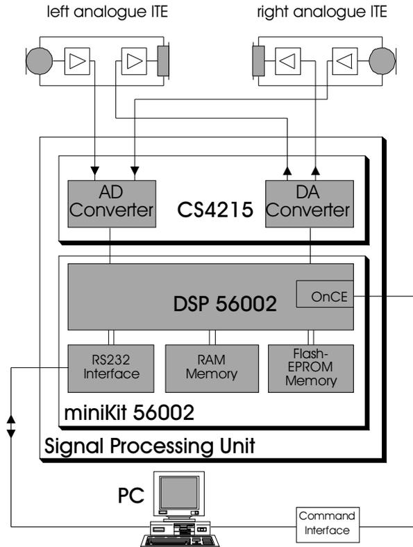
**Figure A.2:** Block diagram of the DASI-2. Algorithms and parameters are downloaded by a PC. Two ITE hearing-aids are used for the in- and output of the acoustical signal.
