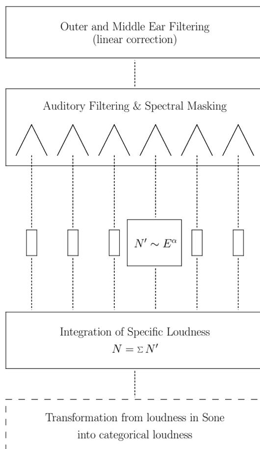
**Figure 4.2:** General structure of a loudness model based on the loudness model proposed by Zwicker. It consists of a fixed filter representing the transfer through the outer and middle ear, calculation of an excitation pattern, transformation of the excitation level into specific loudness and integration of the specific loudness to the total loudness in sone and optionally a transformation into other loudness scales.
