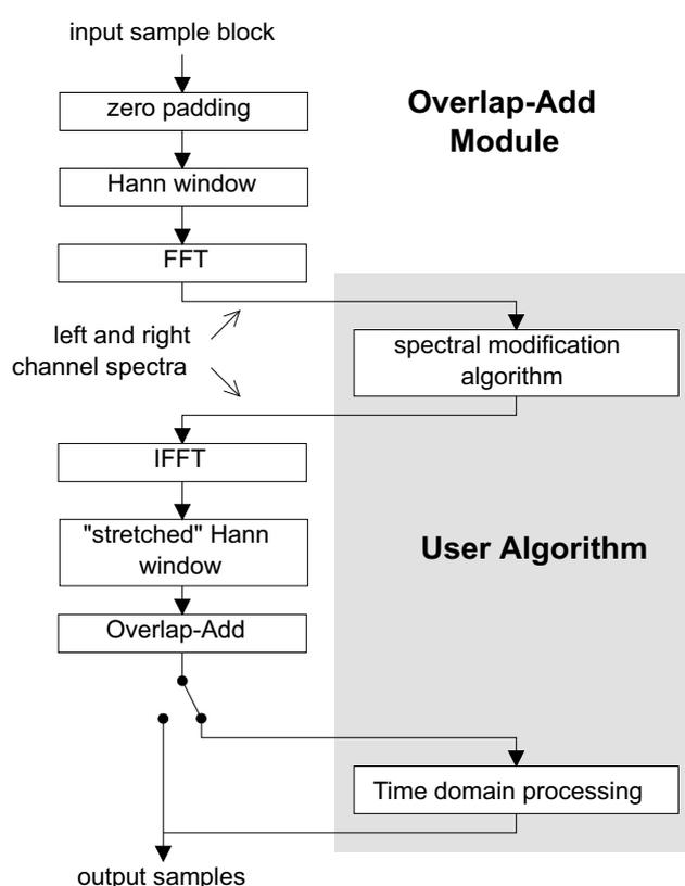
**Figure A.3:** Block diagram of the Overlap–Add framework.
