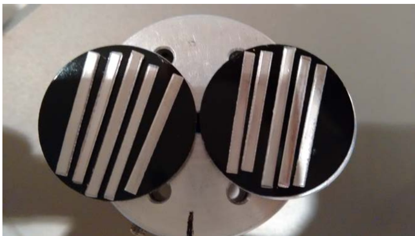
Figure 7-9 – The SEM and EDX samples of stainless steel from the glass cell.
