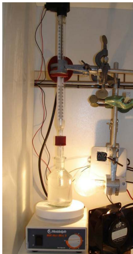
Figure 4-6 – The schematic drawing of the apparatus for the solubility measurement of amorphous silica at 25°C is shown.
