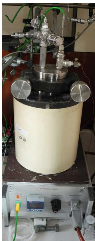
Figure 4-7 – The high pressure and temperature apparatus used for the solubility measurements for the liquid phase and detection of vapour phase silicic acid at 60-170°C and pH-values of 7, 12, and 13.
