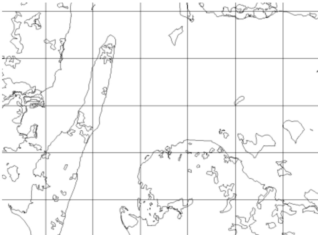
*Figure 2.5: Map of roughness change lines around the Vindeby and Omø Stålgrunde sites; the distance between the grid lines is 10km; roughness values used: 0.0m for water, 0.05m for agricultural areas and 0,4m for cities and forests*
