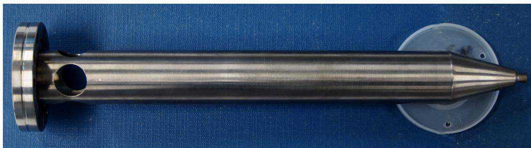
Figure 3.7: Shielding of the mass spectrometer to reduce background contribution to the recorded spectra. The mass spectrometer is mounted on the CF-flange on the left with the ionization source and massfilter within the shielding. The openings on the left are for differential pumping of the spectrometer.
