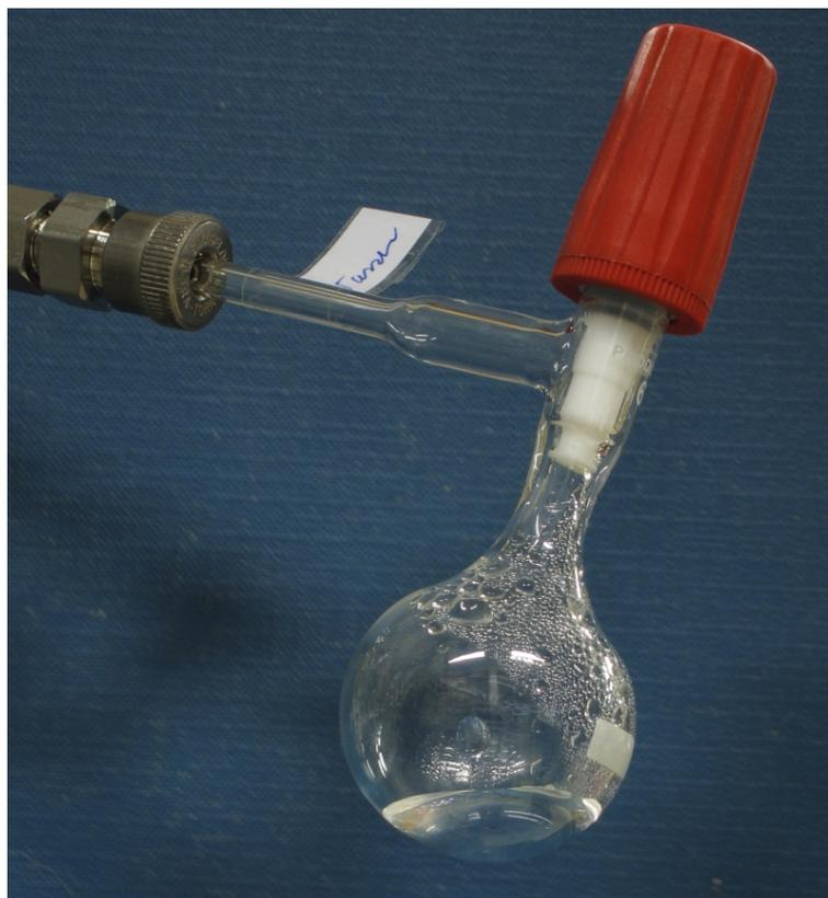
Figure 3.6: A glass flask used for dosing liquids. After freeze-pump-thaw-cycles the flask only contains the liquid and its vapor.
