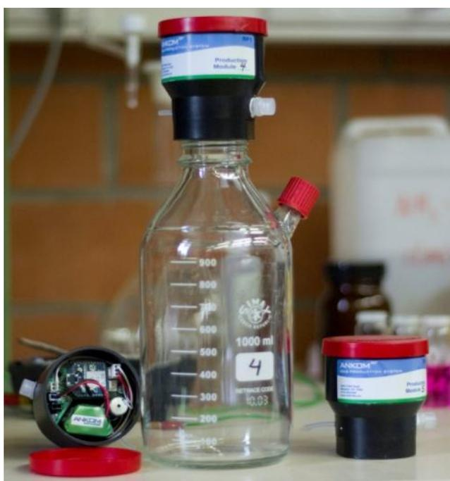
**Figure 9. ANKOM wireless gas production system.**
