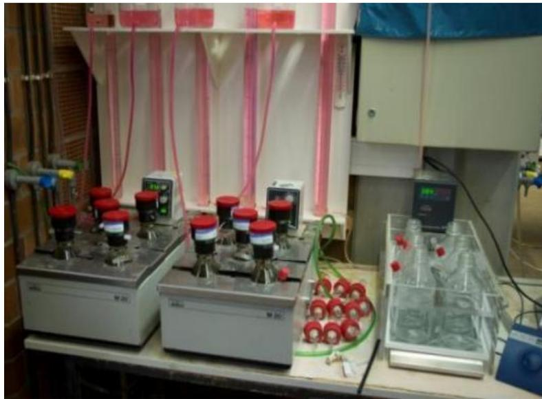
Figure 10. Water baths used for conducting anaerobic digestion experiments.
