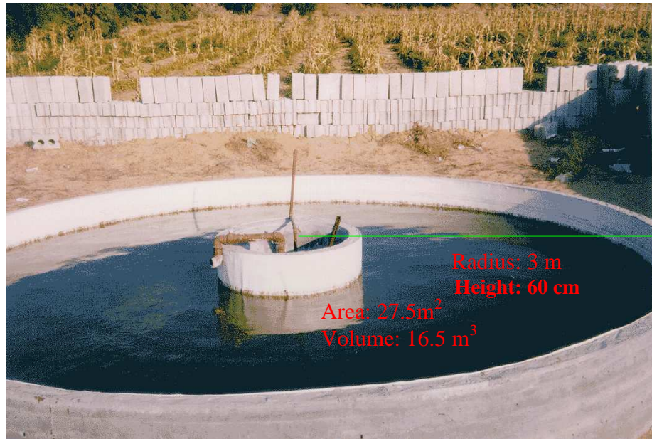
Figure 2.6a. Reference pond at EPRI (Gaza) inoculated with microbial mats from Wadi Gaza. It is used as a reservoir for freshly developed uncontaminated microbial mats for biodegradation experiments.
