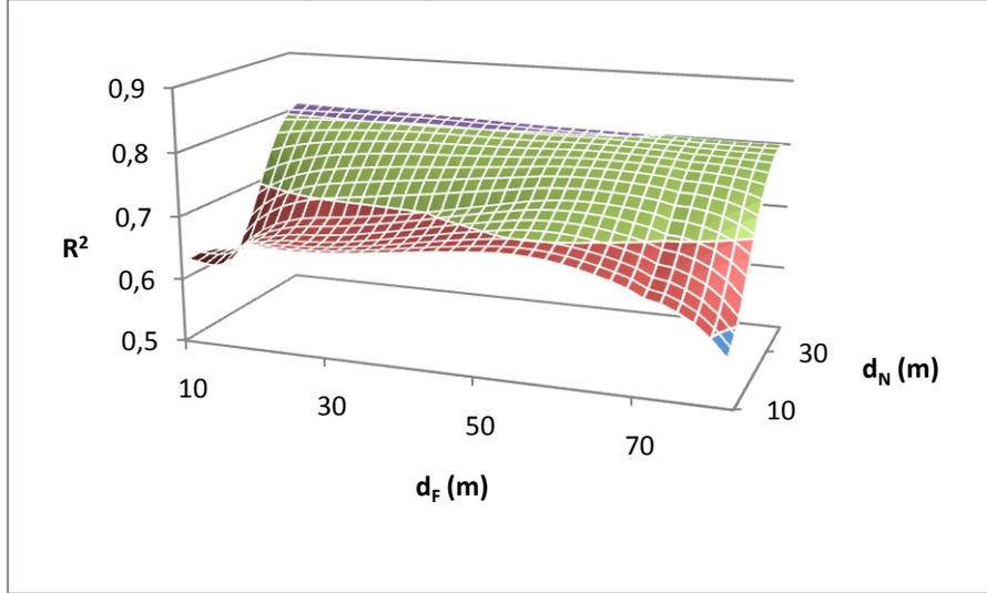
FIGURE 2.1. Coefficient of determination  $R^2$  for multiple regressions on varying distances  $d_N$  and  $d_F$  using the original unmodified 3-parameter S&G lateral control model.
