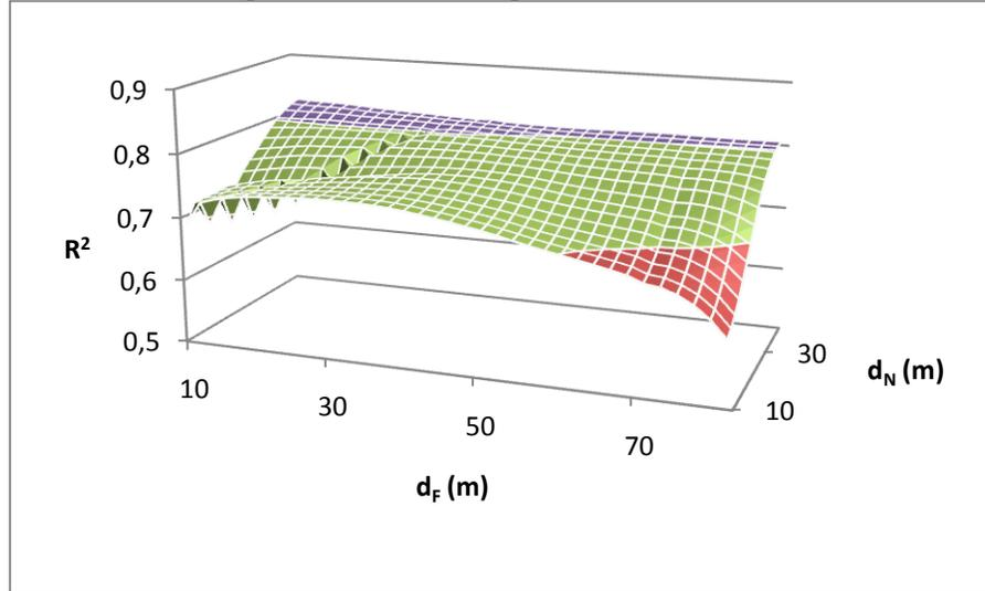
FIGURE 2.2. Coefficient of determination  $R^2$  for multiple regressions on varying distances  $d_N$  and  $d_F$  using the modified lateral control model with segmentation.
