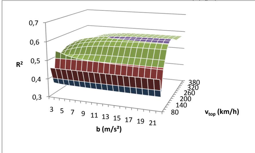
FIGURE 3.1. Coefficient of determination  $R^2$  for multiple regressions on varying distances  $b$  and  $v_{top}$  using the longitudinal control model.
