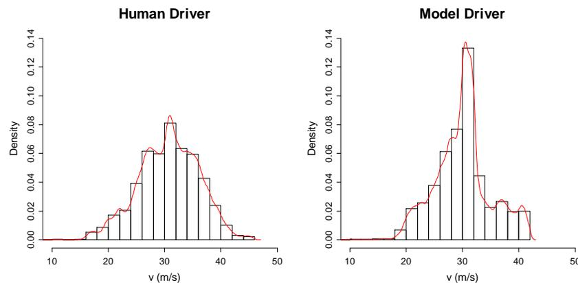
FIGURE 3.2. Density of achieved velocities by Human Driver (left) and integrated model (right) while driving.
