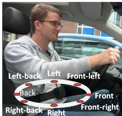
Figure 5.4: Vibrators location on the tactile belt used in experiments.
