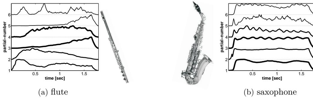
Figure A.6: Amplitude line spectrogram for the first 6 harmonics in the flute (a) and saxophone (b) sounds. Displayed are the envelopes of the harmonics normalized to the respective harmonic maxima. Thick lines indicate partials which dominate the mean spectrum, or those, with the higher mean amplitude.
