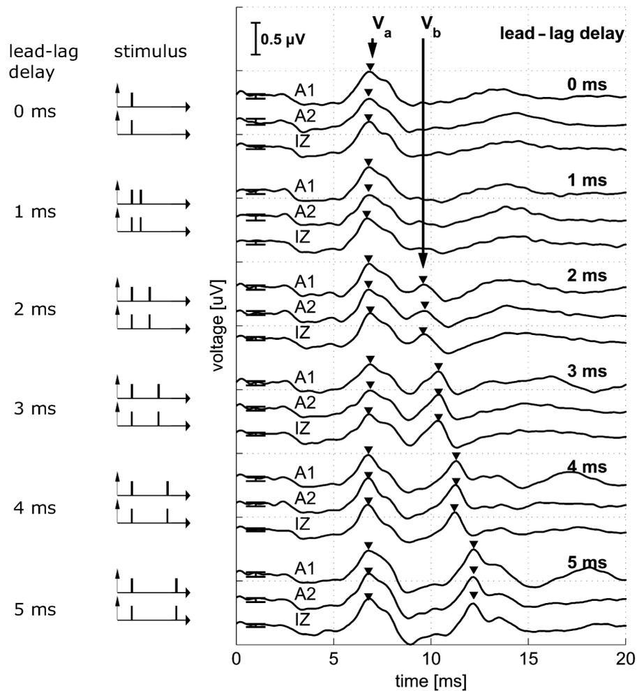
**Fig. 4.4:** **Left panel:** Sketch of the time signals used for the ABR recordings in Experiment I (diotic stimulation) with increasing lead-lag delay (0 ms to 5 ms). **Right panel:** Corresponding ABRs of subject S1. Potentials of three channels (A1, A2 and IZ) are shown for each lead-lag delay. Errorbars at a latency of 1 ms indicate the intraindividual standard error.
