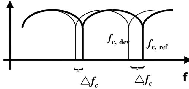
Fig. 2.8: Illustration of the spectra of reference (thick line) and deviant (thin line). Due to comb filter effects frequencies  $f_{c, std}$  cancel in the spectrum of the reference and frequencies  $f_{c, dev}$  cancel in the spectrum of the deviant in dependence of the lead-lag delay and the lag-ITD. In addition, differences  $\Delta f_c$  between the notch frequencies in the spectra of reference and deviant stimulus are indicated.
