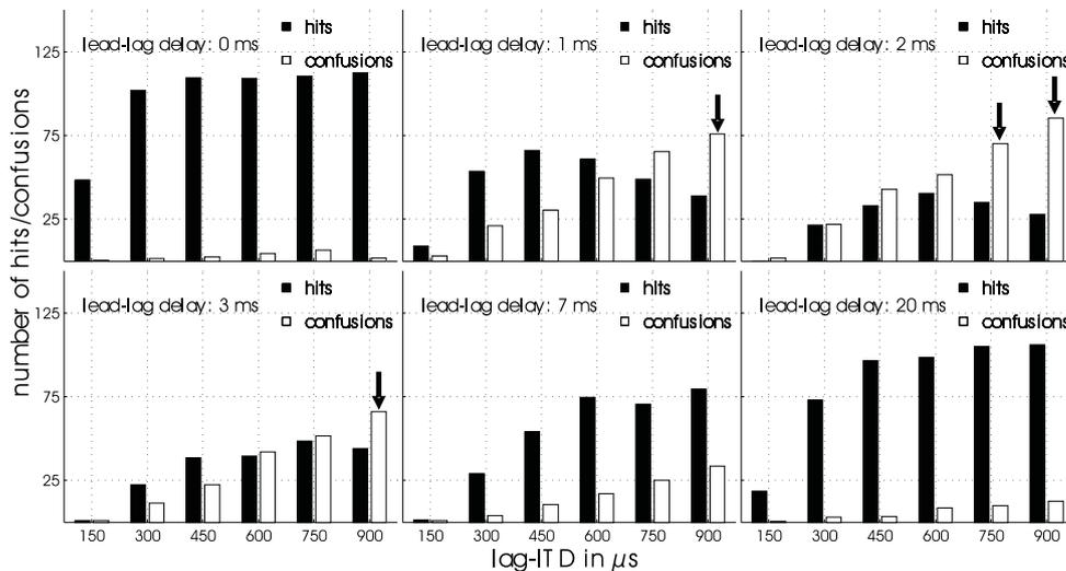
Fig. 3.8: Illustration of hits (filled bars) and direction confusions (open bars) that occurred in the 'pick-out' experiment in dependence on the lag-ITDs and lead-lag delays. Data were accumulated across eight subjects. Mean hits and mean direction confusions of lateralizations to the left and right hand side are shown. Arrows indicate those number of direction confusion values that are significantly larger than the corresponding number of hit values.
