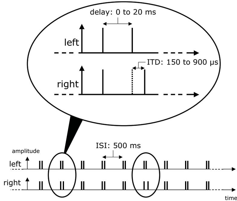
Fig. 2.3: Sketch of the stimulus sequence used in Experiment V ('pick-out'). The sequence overall consisted of about 210 lead-lag click-pairs (about 180 reference stimuli and 30 deviants). The interaural time difference of the lag click of the deviant, see enlarged cut-out, was varied from 0  $\mu\text{s}$  up to 900  $\mu\text{s}$  in steps of 150  $\mu\text{s}$ . The lead-lag delay was varied from 0 ms up to 20 ms. Within one sequence the lead-lag delay is kept constant.
