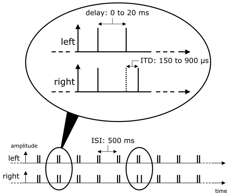
Fig. 3.3: Sketch of the stimulus sequence as used in the 'pick-out' experiment (Experiment III). Overall, the sequence consisted of about 210 lead-lag click-pairs. The interaural time difference of the lag click of the deviant, see enlarged cut-out, was varied from 0  $\mu\text{s}$  up to  $\pm 900 \mu\text{s}$  in steps of  $\pm 150 \mu\text{s}$ . The lead-lag delay was varied from 0 ms up to 20 ms. Within one sequence the lead-lag delay was kept constant.
