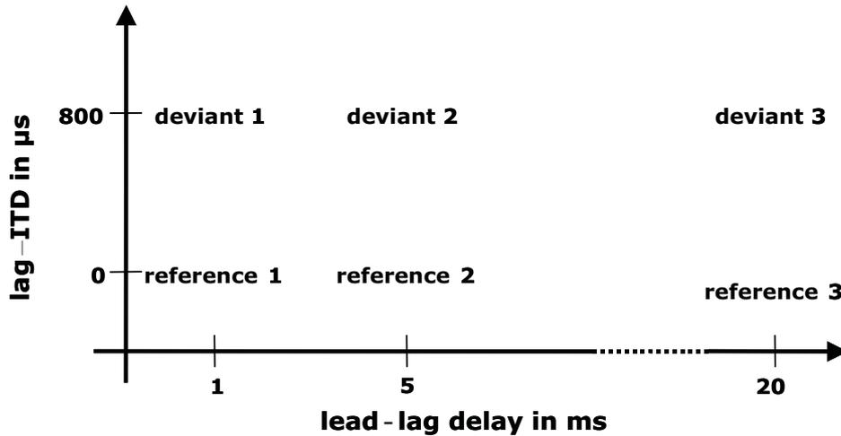
Fig. 4.3: Overview of the stimulus parameters that were applied for the CAEP recordings. Lead-lag delays of 1, 5 and 20 ms were used. Within a stimulus sequence the lead-lag delay was fixed. For each lead-lag delay the reference stimuli had a lag-ITD of 0  $\mu\text{s}$  and the deviants had a lag-ITD of 800  $\mu\text{s}$ .
