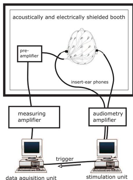
Fig. 4.1: Sketch of the EEG recording setup. Stimuli were presented via insert-ear phones. The EEG was recorded from 31 or 3 electrodes, respectively.
