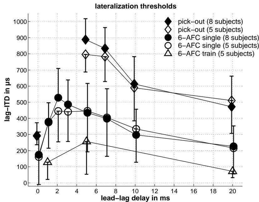
Fig. 3.4: Lateralization thresholds obtained by Experiment I ('3-I 6-AFC single', circles), Experiment II ('3-I 6-AFC train', triangles) and Experiment III ('pick-out', diamonds). Lag-ITDs that yield 70.7 percent correct performances were plotted as a function of the lead-lag delay. Open symbols show data averaged across those five subjects that participated in all experiments, closed symbols show data averaged across eight subjects. Errorbars indicate interindividual standard deviations.
