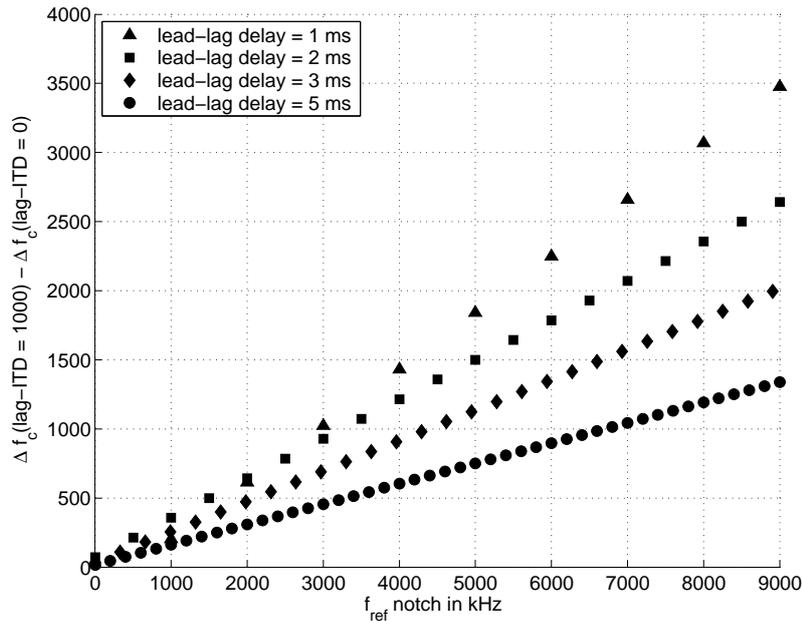
Fig. 2.10: Plot of the difference between the  $\Delta f_c$ s obtained with a lag-ITD of  $1000 \mu\text{s}$  and  $0 \mu\text{s}$  versus the cancelled frequency of the reference stimulus. Triangles, squares, diamonds and circles represent lead-lag delays of 1, 2, 3 and 5 ms, respectively.
