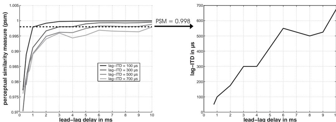
Fig. 2.11: **Left panel:** Plot of the perceptual similarity measure (PSM) for different lag-ITDs as a function of the lead-lag delay. **Right panel:** Plot of the lag-ITD for a constant PSM of 0.998.
