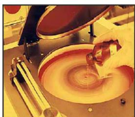
**FIGURE 5.2:** Spin coating is the wide spread option for obtaining organic thin films
